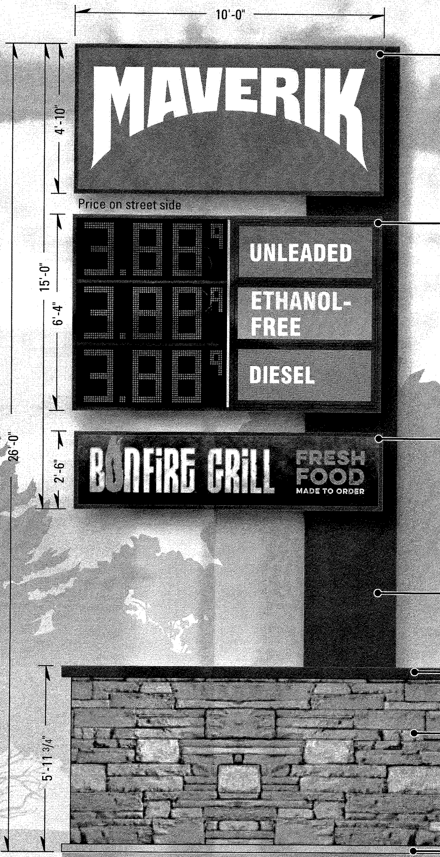
1 D/F ILLUMINATED PYLON SIGN
