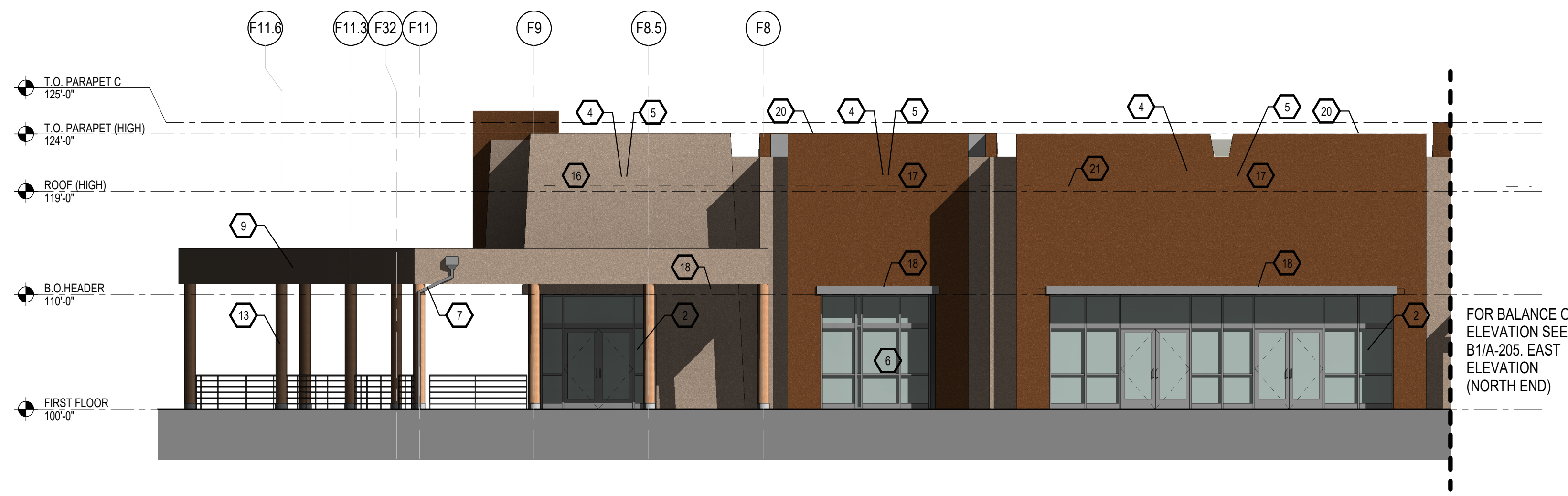
A1 EAST BUILDING ELEVATION (SOUTH END) 1/8" = 1'-0"
