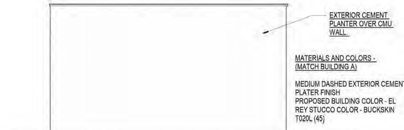
B2 TRASH - SIDE ELEVATION 3/8" = 1'-0"
