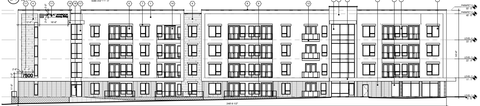
A1 WEST ELEVATION - BUILDING A Scale: 3/32" = 1'-0"
