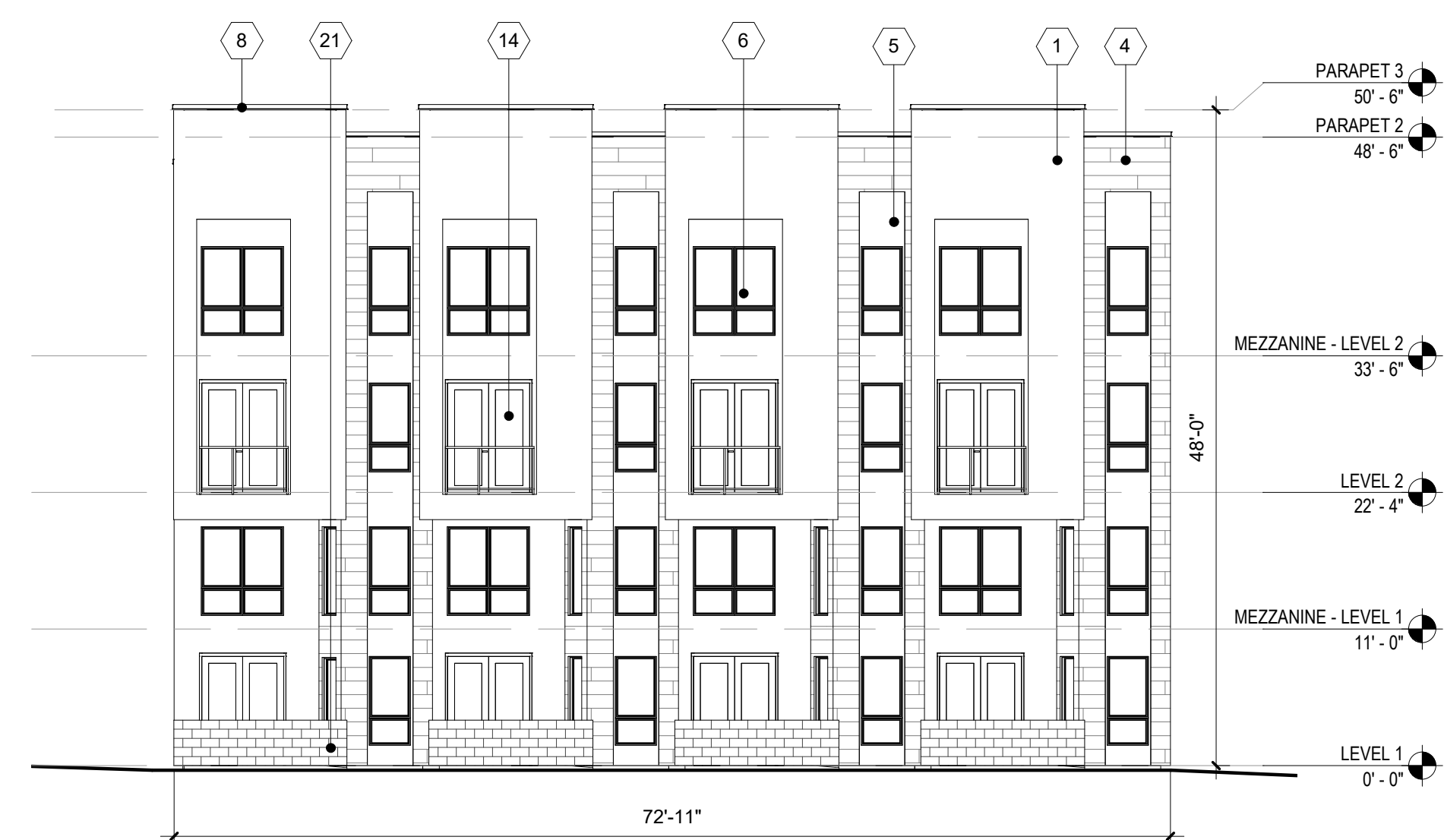
C1 NORTH ELEVATION - BUILDING C Scale: 3/32" = 1'-0"
