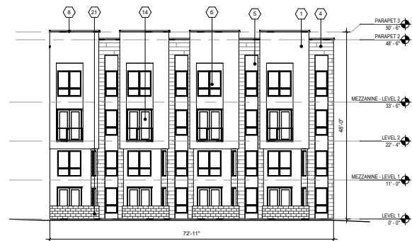
C1 NORTH ELEVATION - BUILDING C Scale 3/32" = 1'-0"
