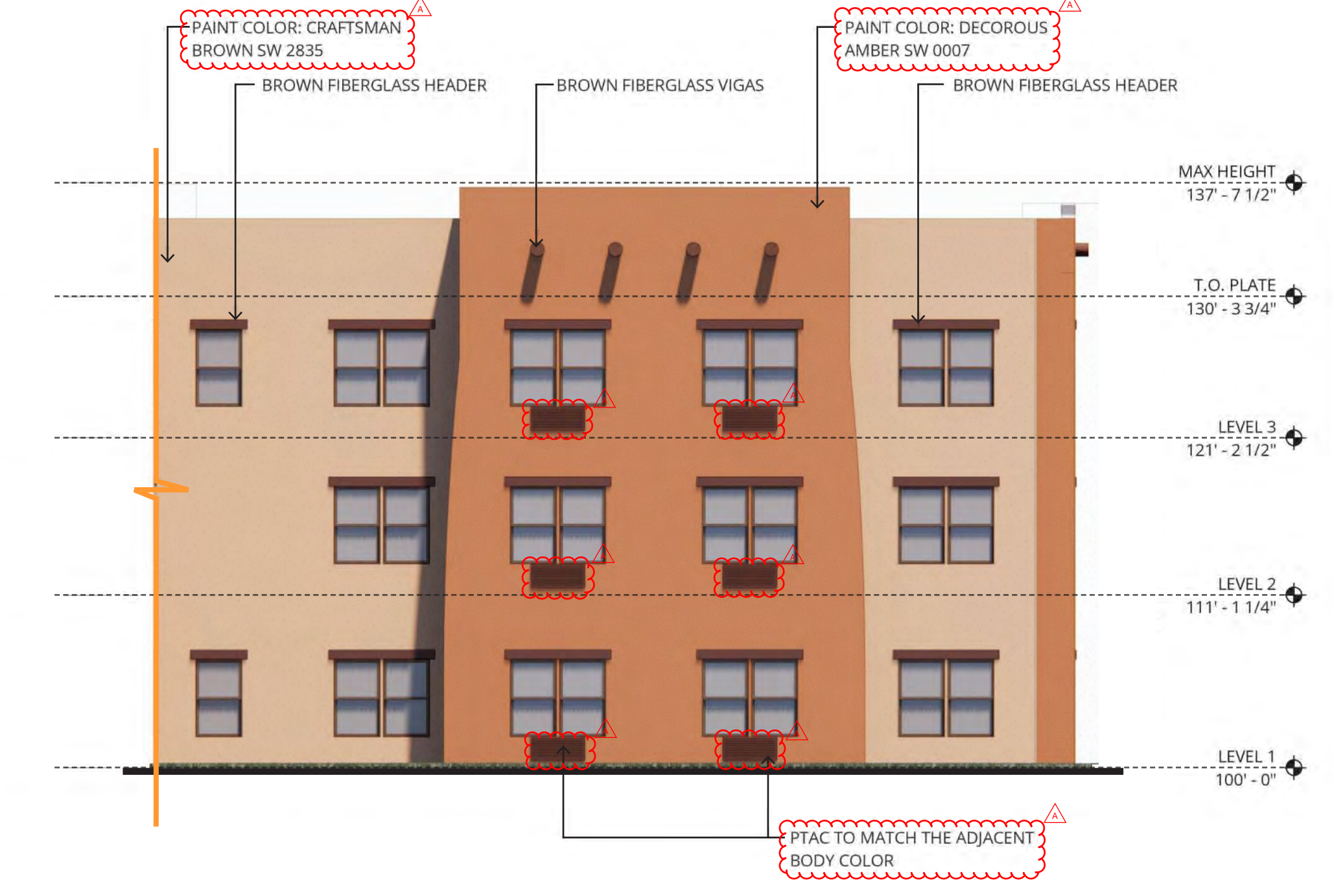
4 PARTIAL NORTH ELEVATION - AL WING - A 1/8" = 1'-0"
