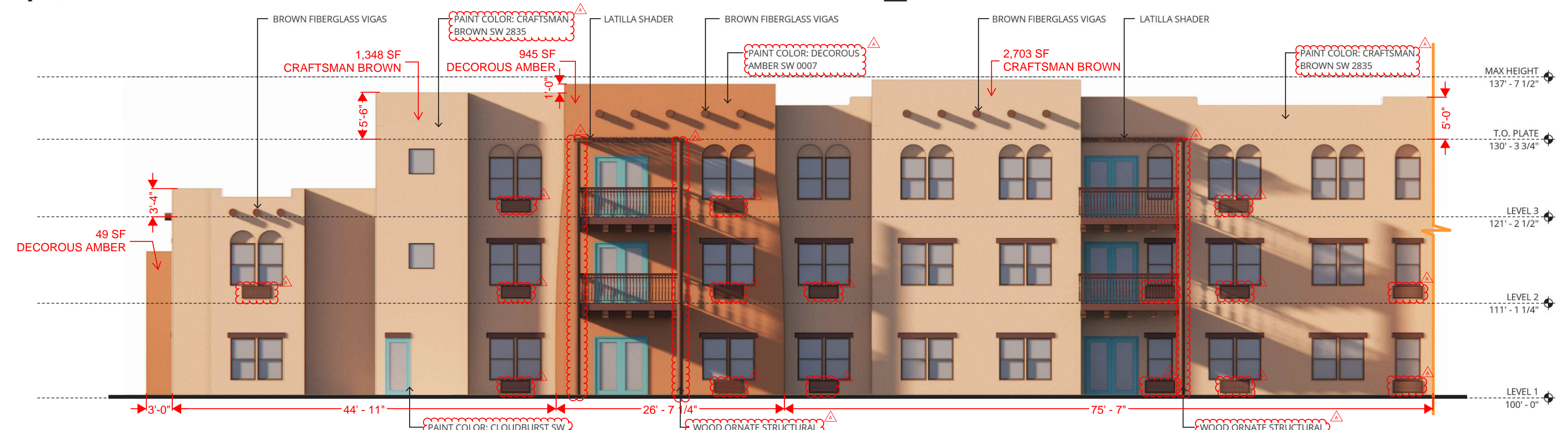
3 EAST ELEVATION - AL WING 1/8" = 1'-0"
