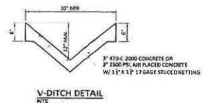
V-DITCH DETAIL NTS
