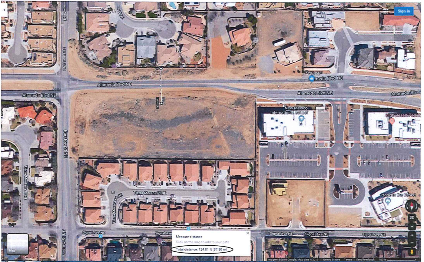
Figure 9: True 124-foot "Right of Way" lines up Property Lines, Sidewalks, Median and Street
