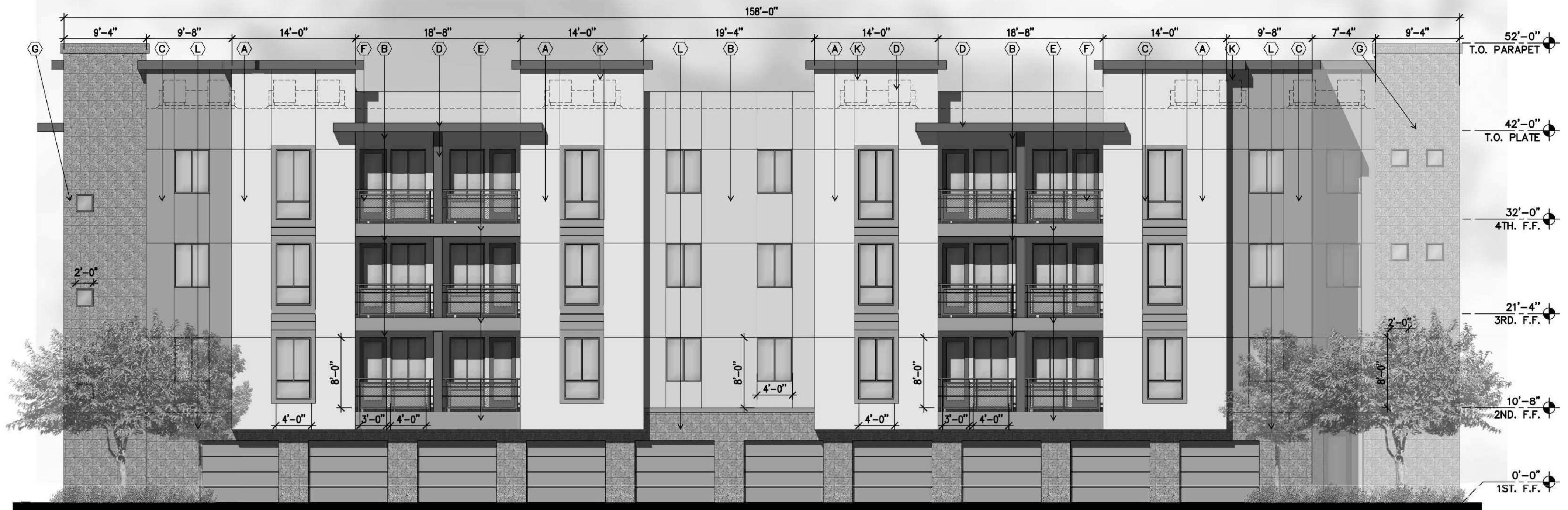
BLDG. TYPE 2 FRONT ELEVATION
