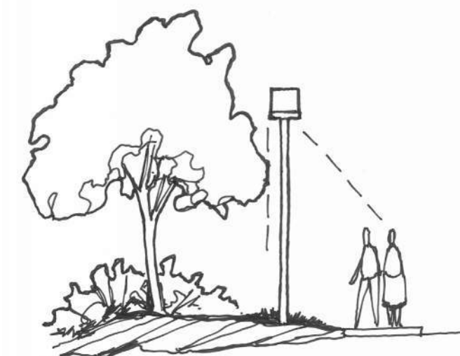
LIGHTING - should be shielded source, with the height kept to a minimum necessary to meet safety standards
