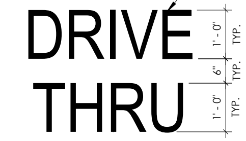
D5 PAVEMENT MARKING - TWO LINES 1/2" = 1'-0"
