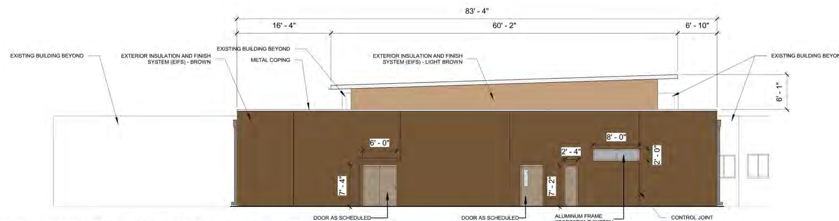
B1 BUILDING ELEVATION - EAST (PHASE 1) 1" = 10'-0"
