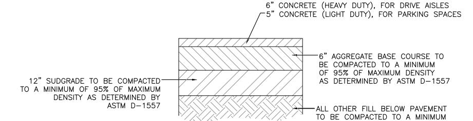
TYPICAL PAVING SECTION MATERIAL DESIGNATION FOR CONCRETE AND AGGREGAT BASE
