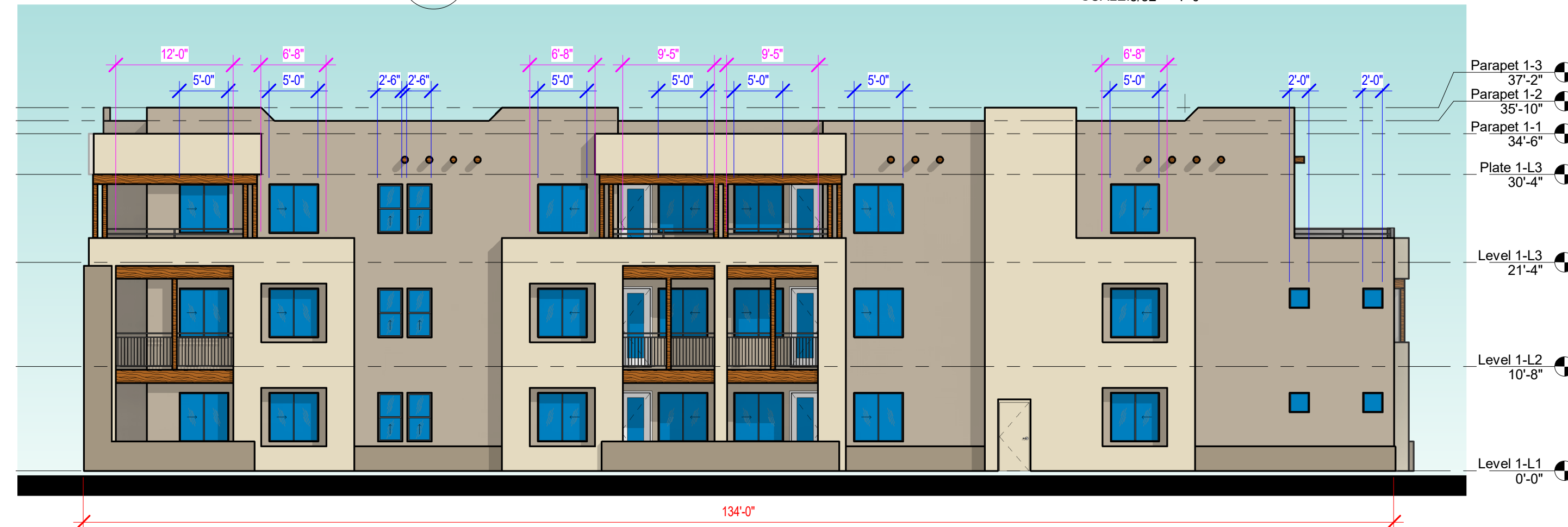
3 BLDG 1 - EAST ELEVATION SCALE: 3/32" = 1'-0"
