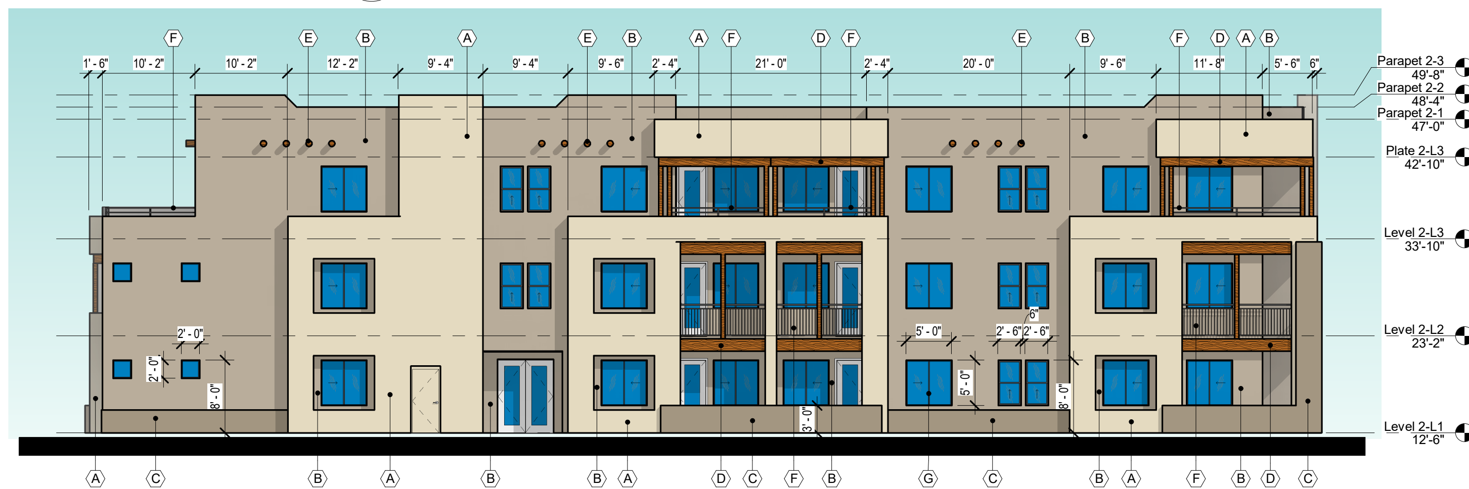
2 BLDG 2 - WEST ELEVATION SCALE: 3/32" = 1'-0"
