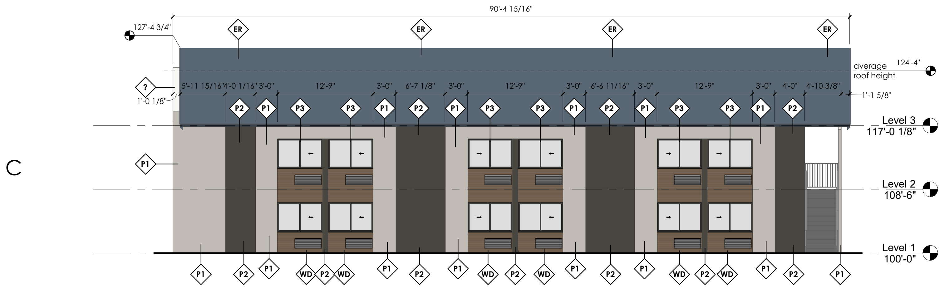
C1 BUILDING 3 - ELEVATION EAST 1/8" = 1'-0"
