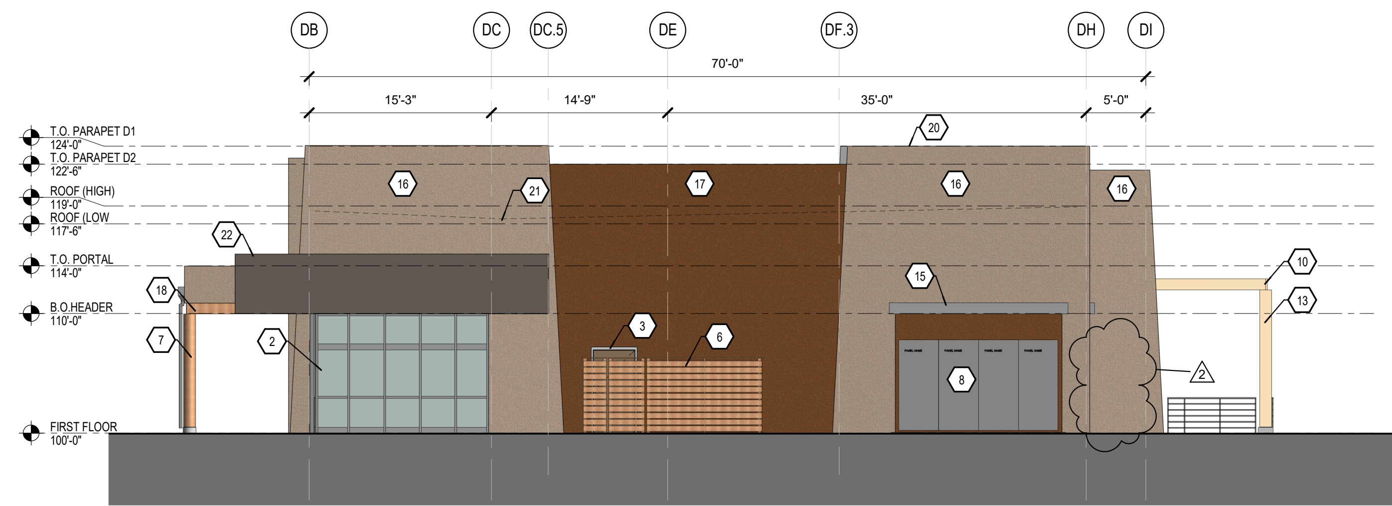
A1 WEST BUILDING ELEVATION 1/8" = 1'-0"
