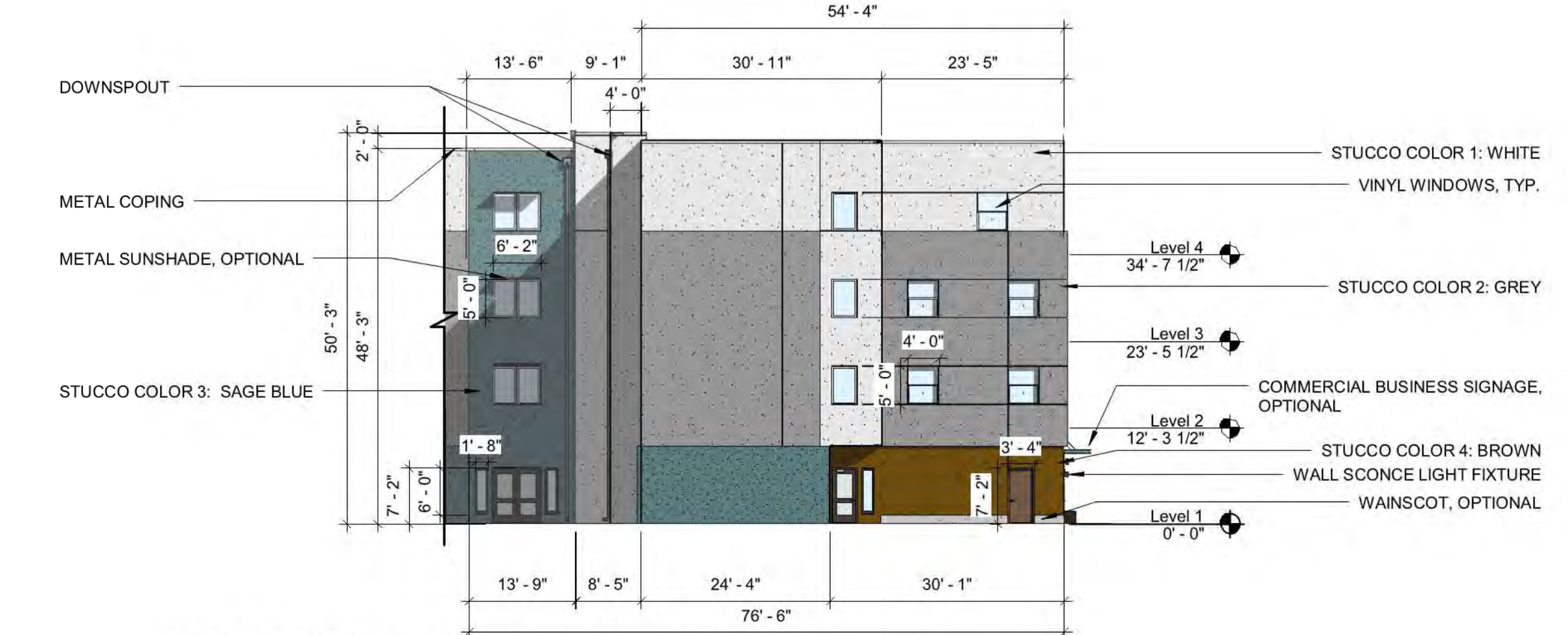
C4 EAST ELEVATION - NORTH END 1/16" = 1'-0"
