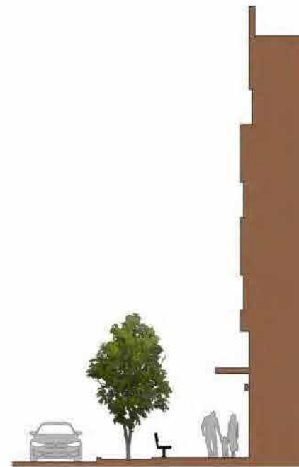
Street section along Central Avenue with commercial uses, landscape buffer with street trees and building lighting, awnings, & street furniture.
