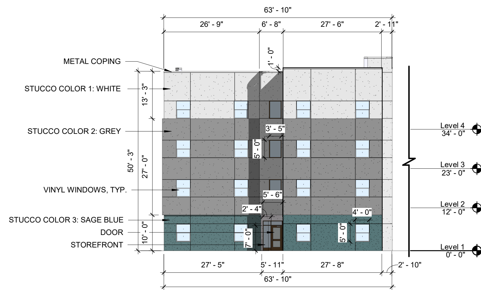
B1 SOUTH ELEVATION - WEST END 1/16" = 1'-0"
