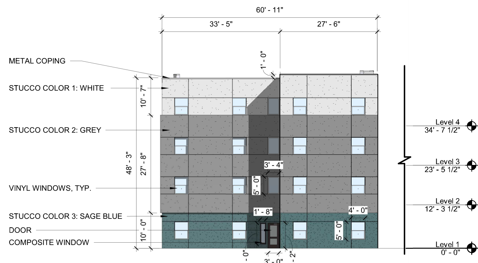
B1 SOUTH ELEVATION - WEST END 1/16" = 1'-0"
