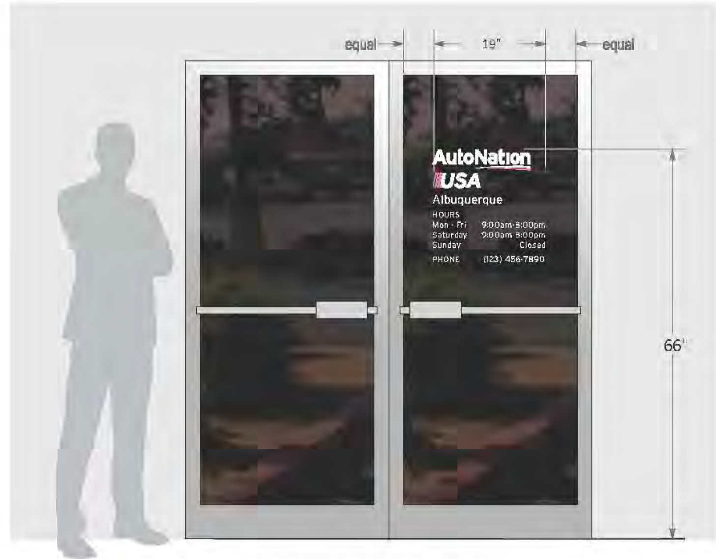
When there are double-Entry doors, the vinyl graphics will be placed on the right door
