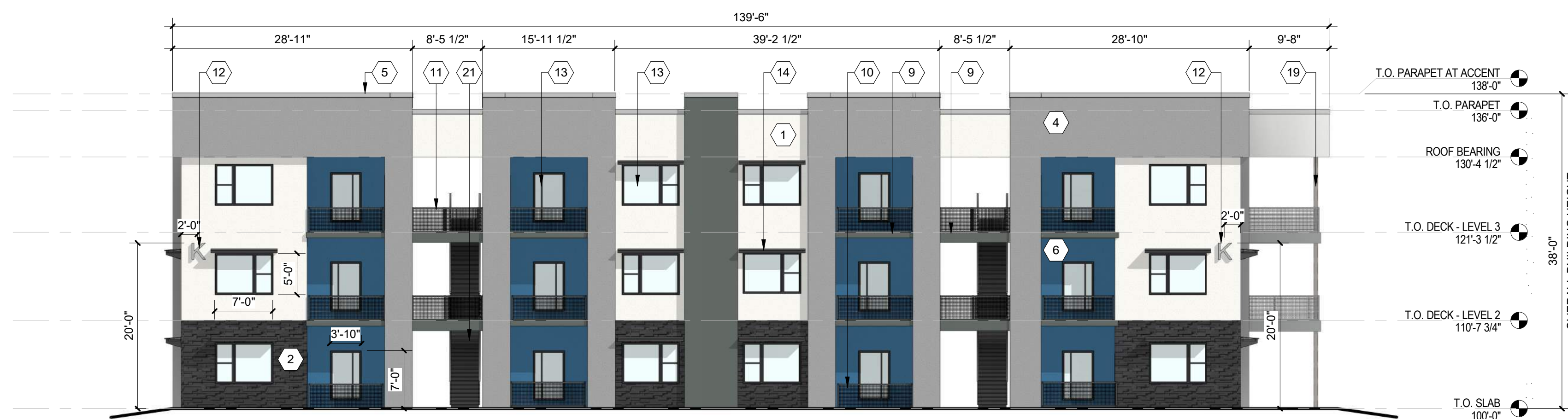
A2 BUILDING K - WEST ELEVATION 3/32" = 1'-0"
