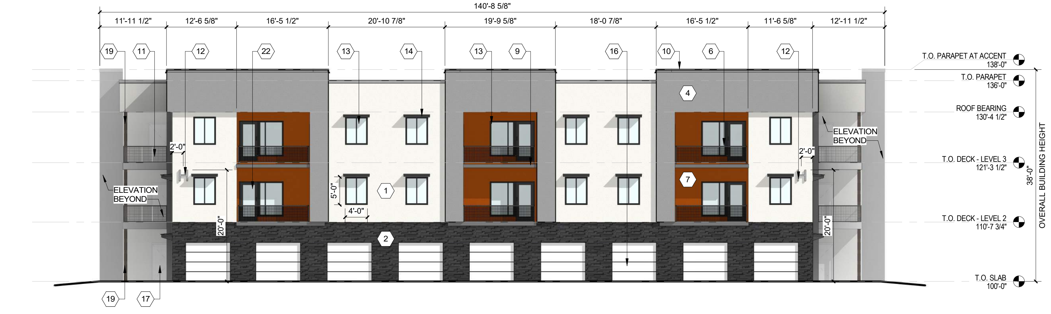
A2 BUILDING H - EAST ELEVATION 3/32" = 1'-0"
