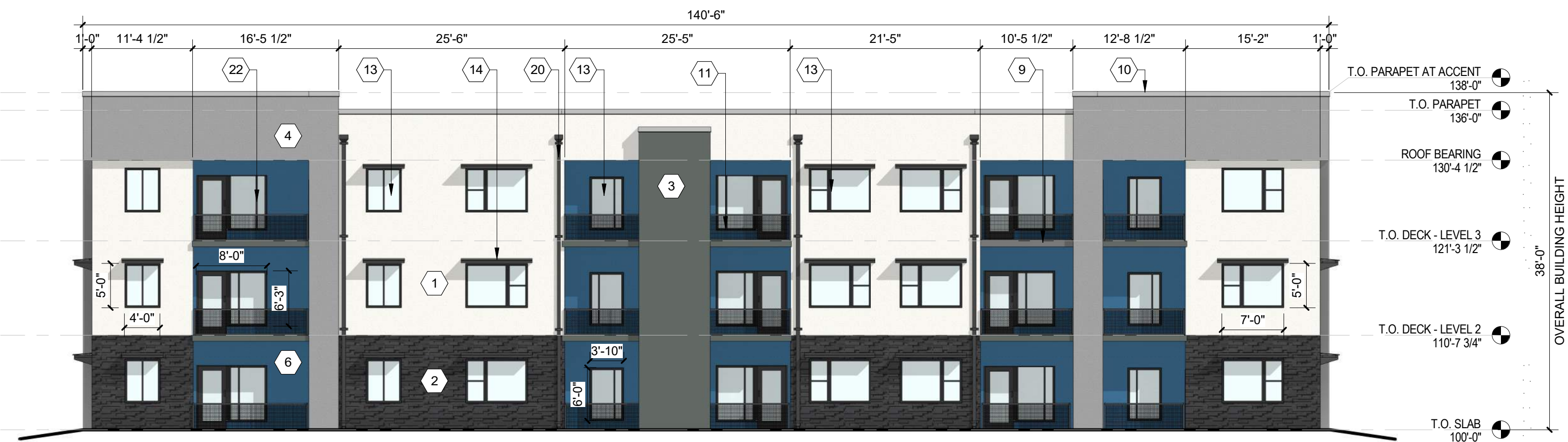
B2 BUILDING K - EAST ELEVATION 3/32" = 1'-0"
