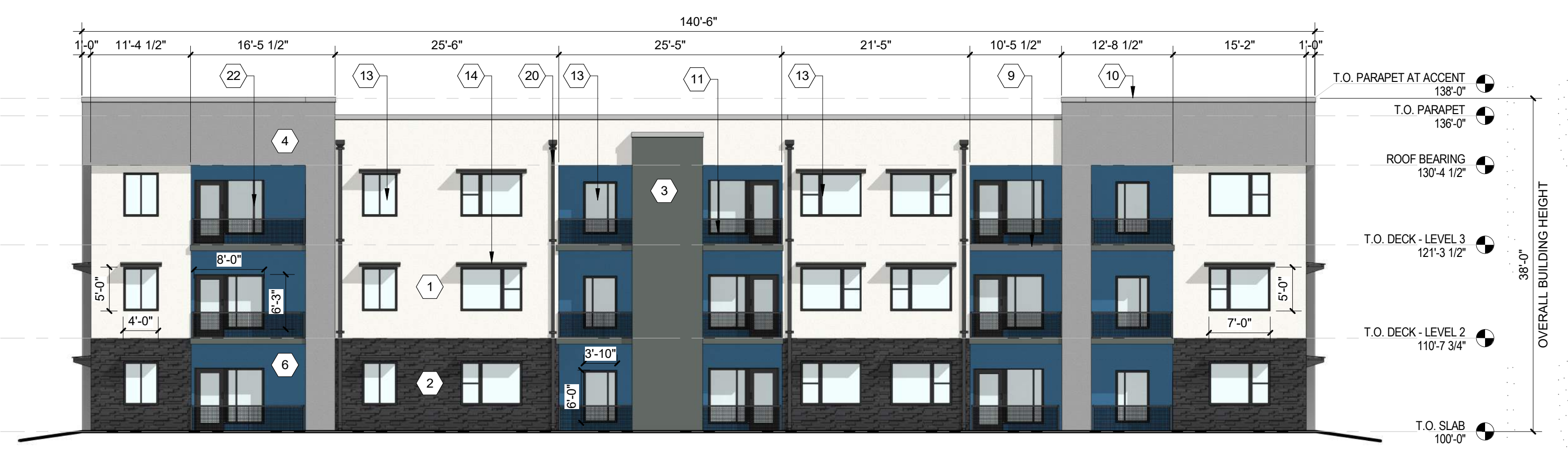
B2 BUILDING K - EAST ELEVATION 3/32" = 1'-0"
