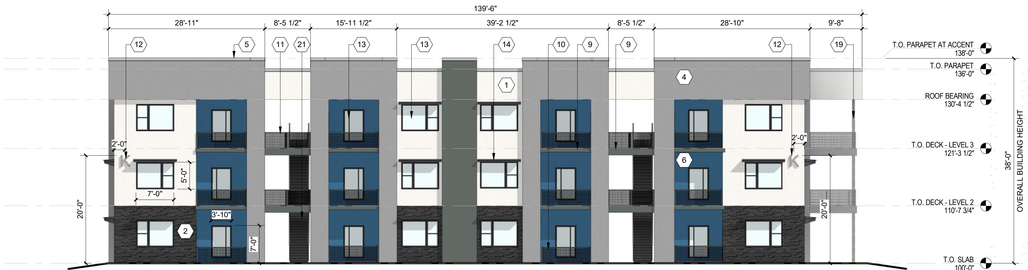
A2 BUILDING K - WEST ELEVATION 3/32" = 1'-0"
