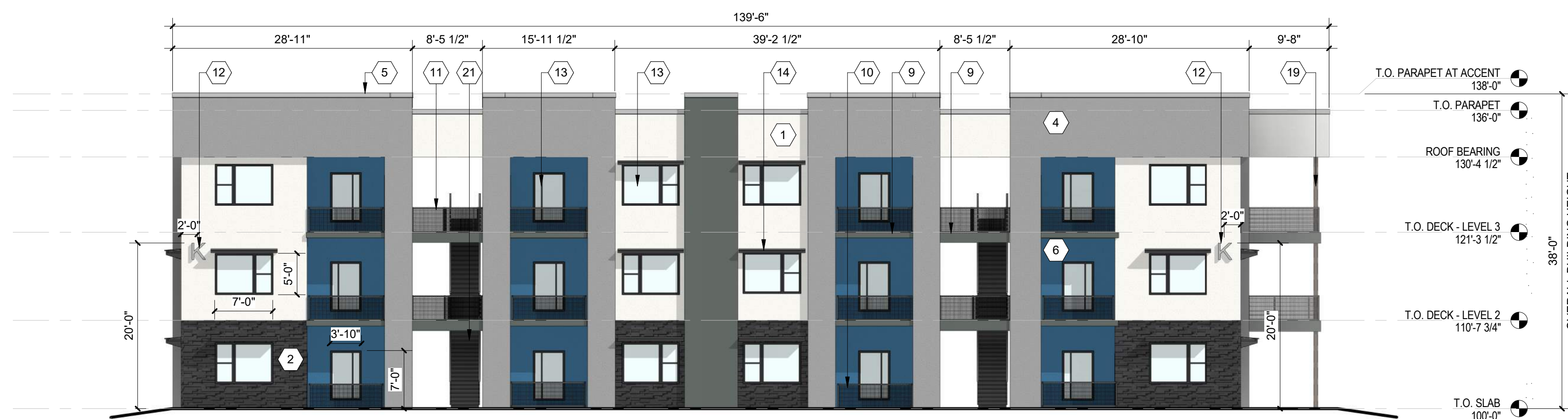
A2 BUILDING K - WEST ELEVATION 3/32" = 1'-0"
