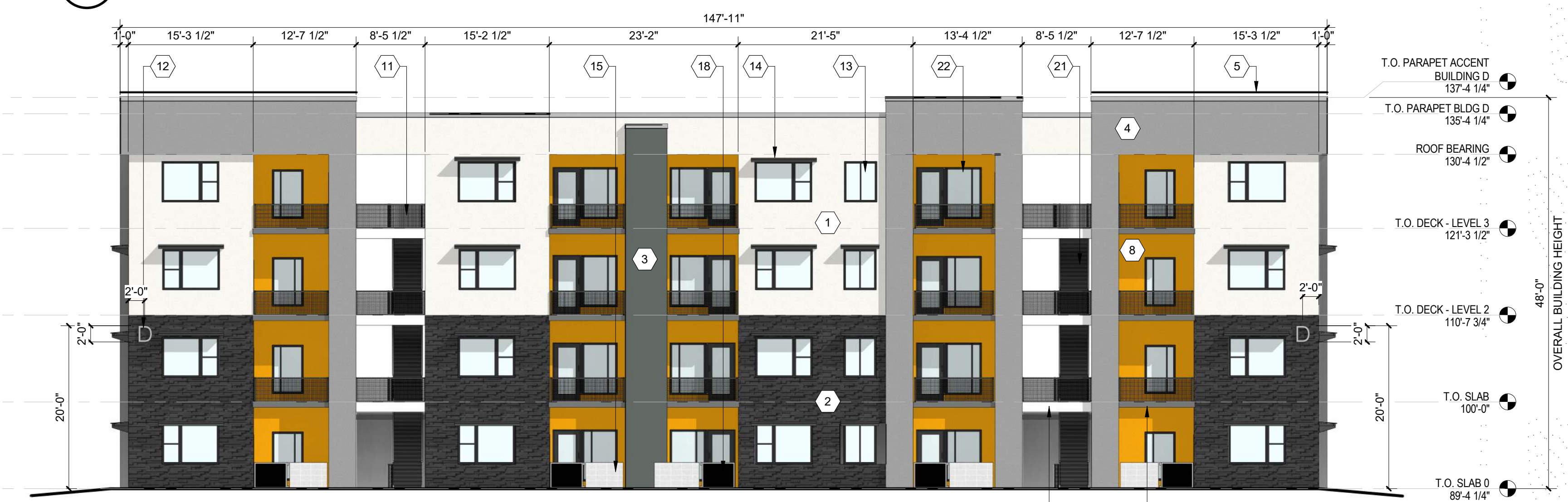
B2 BUILDING D - WEST ELEVATION 3/32" = 1'-0"
