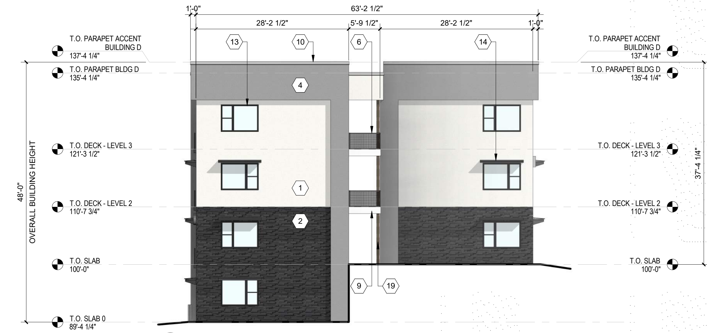
C4 BUILDING D - SOUTH ELEVATION 3/32" = 1'-0"
