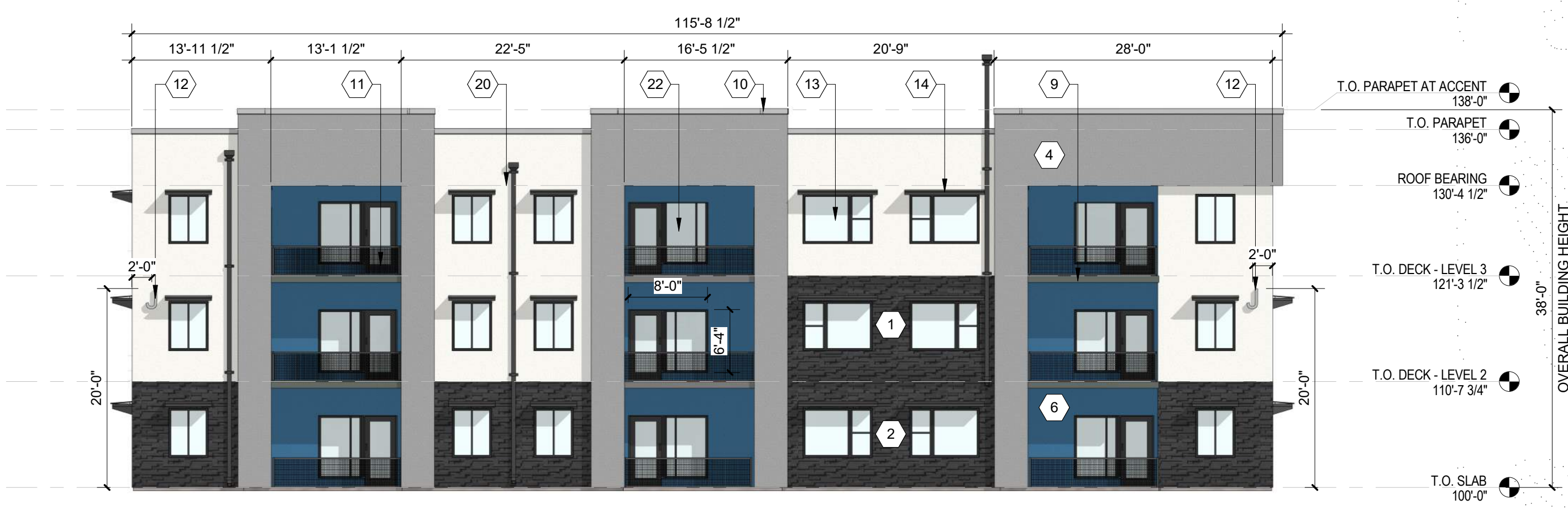
B2 BUILDING J - WEST ELEVATION 3/32" = 1'-0"
