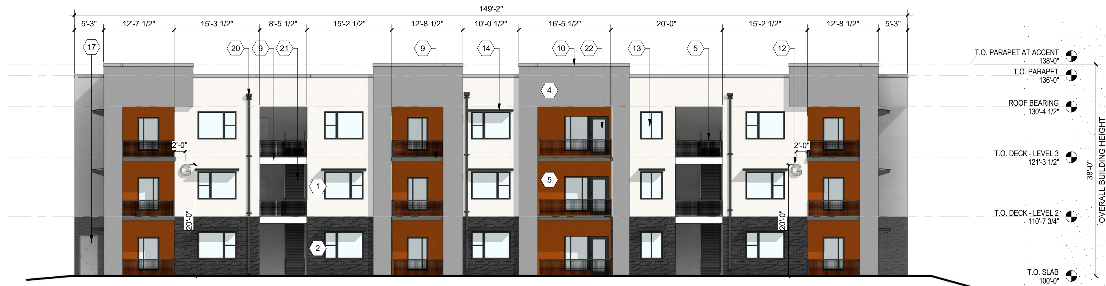
B2 BUILDING G - WEST ELEVATION 3/32" = 1'-0"
