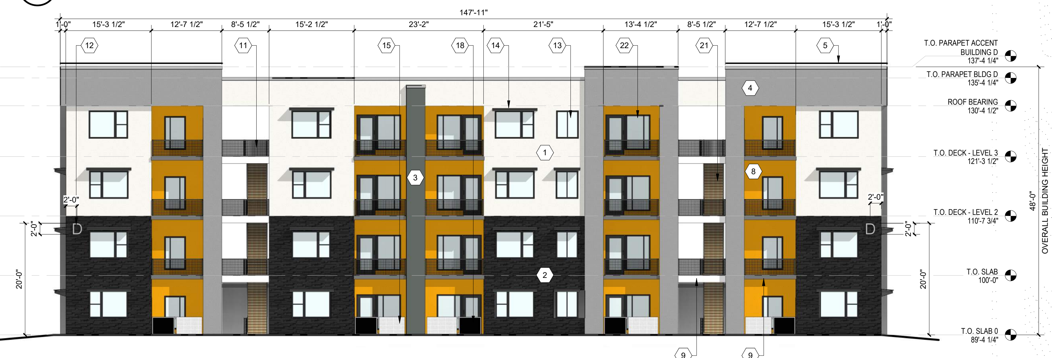
A2 BUILDING D - EAST ELEVATION 3/32" = 1'-0"
