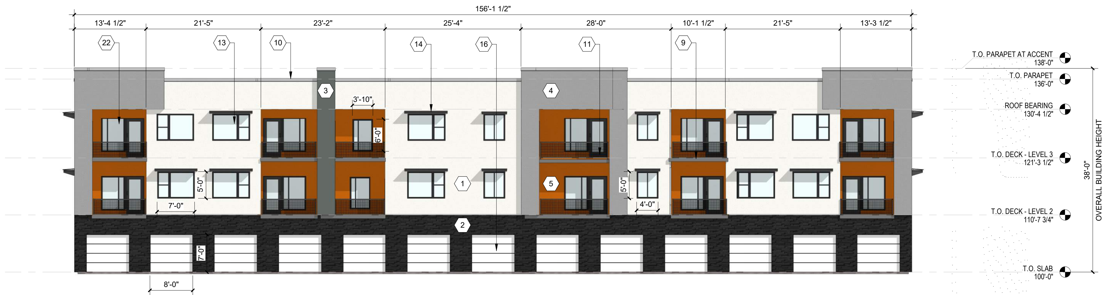
A2 BUILDING F - EAST ELEVATION 3/32" = 1'-0"
