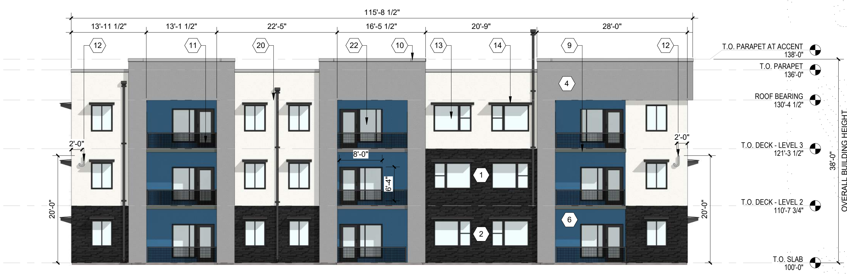
B2 BUILDING J - WEST ELEVATION 3/32" = 1'-0"
