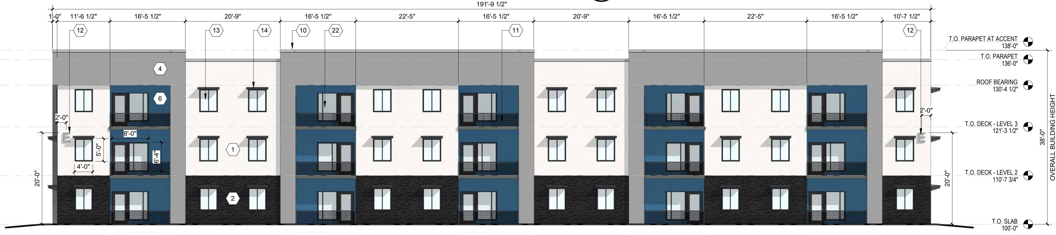
B2 BUILDING E - WEST ELEVATION 3/32" = 1'-0"
