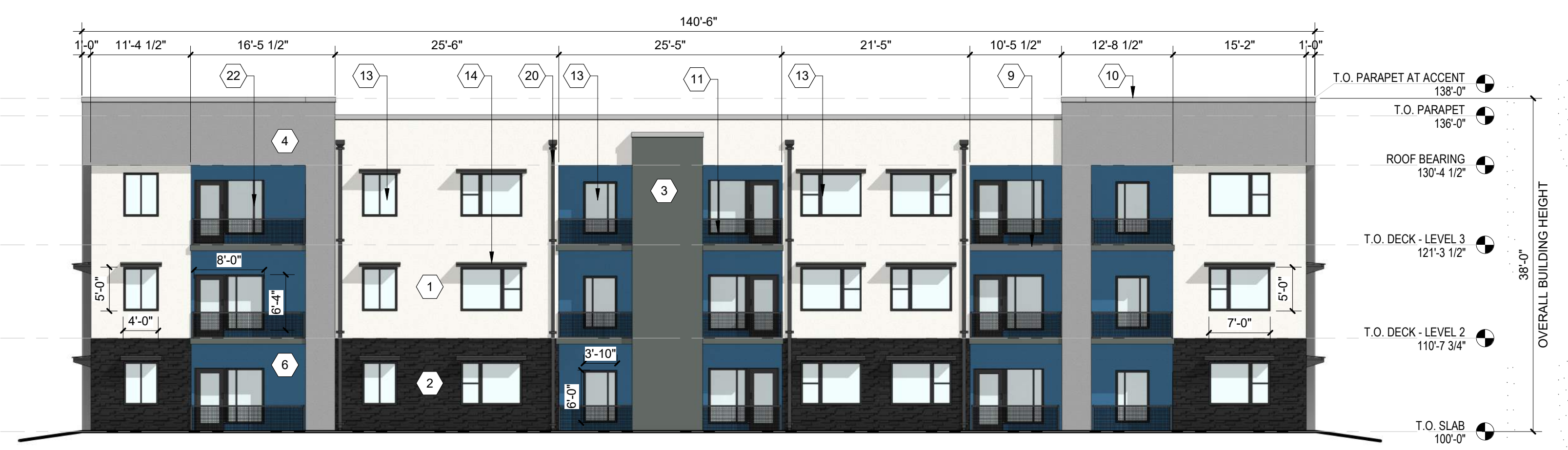
B2 BUILDING K - EAST ELEVATION 3/32" = 1'-0"
