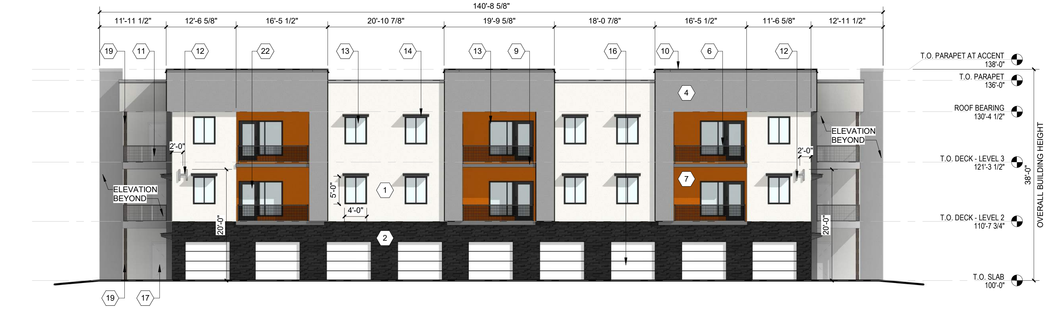
A2 BUILDING H - EAST ELEVATION 3/32" = 1'-0"
