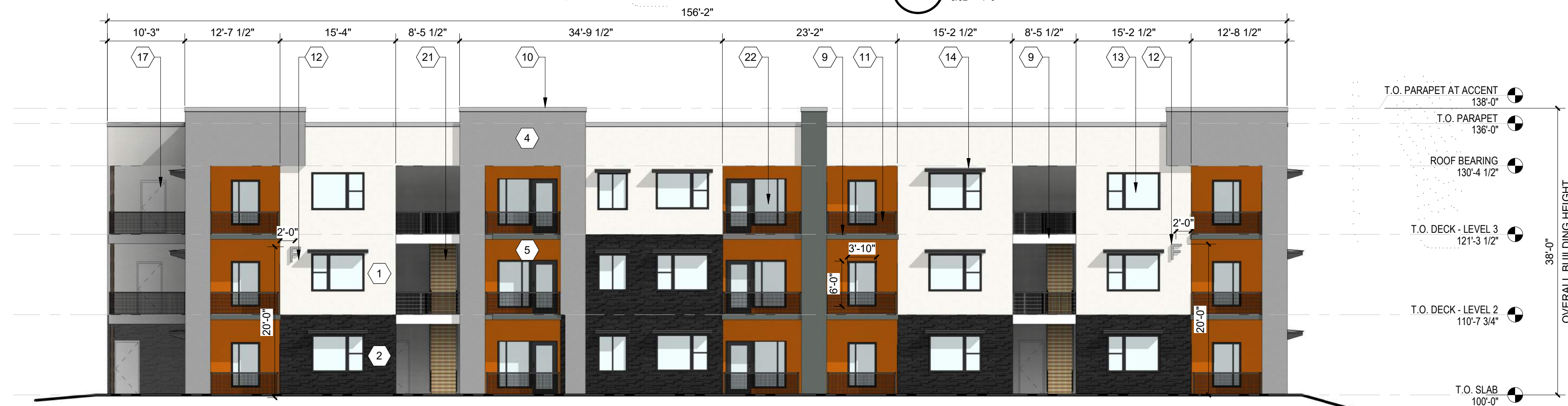
B2 BUILDING F - WEST ELEVATION 3/32" = 1'-0"
