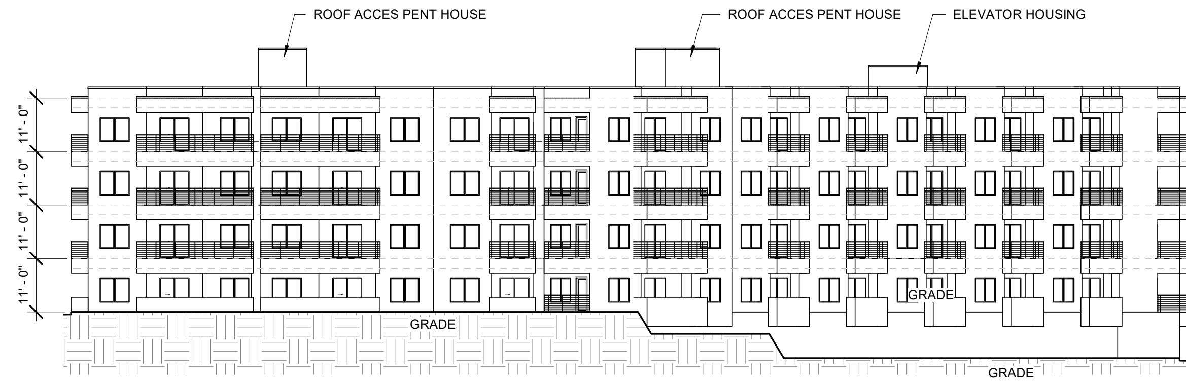
BUILDING 400 EAST ELEVATION
