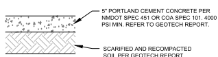
STANDARD DUTY CONCRETE PAVEMENT SECTION FOR TRAFFIC CATEGORY A * CONCRETE FOR RIGID PAVEMENT SHOULD HAVE A MINIMUM 28-DAY COMPRESSIVE STRENGTH OF 4,000 PSI, A MODULUS OF RUPTURE OF 500 PSI, AND BE PLACED WITH A MAXIMUM SLUMP OF 4 INCHES.
