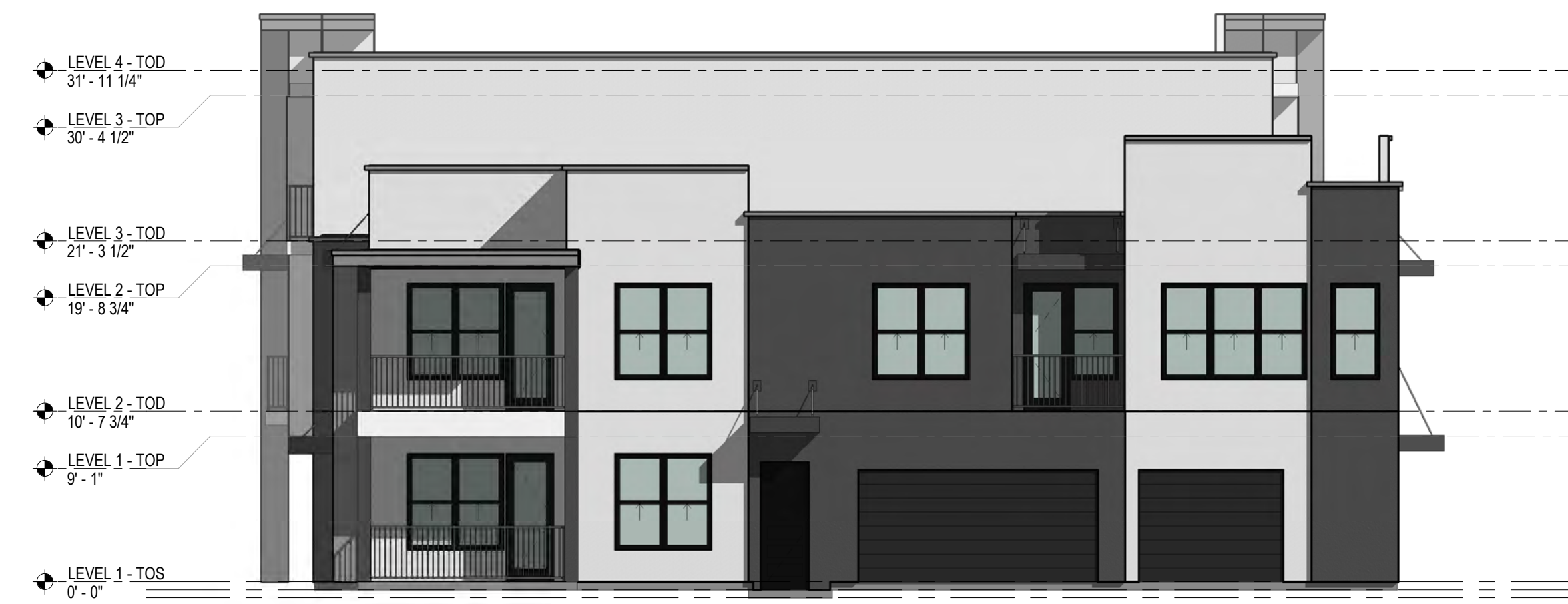
3 DRB - BLDG TYPE II - LEFT ELEVATION 1/8" = 1'-0" 0 2 4 8 16
