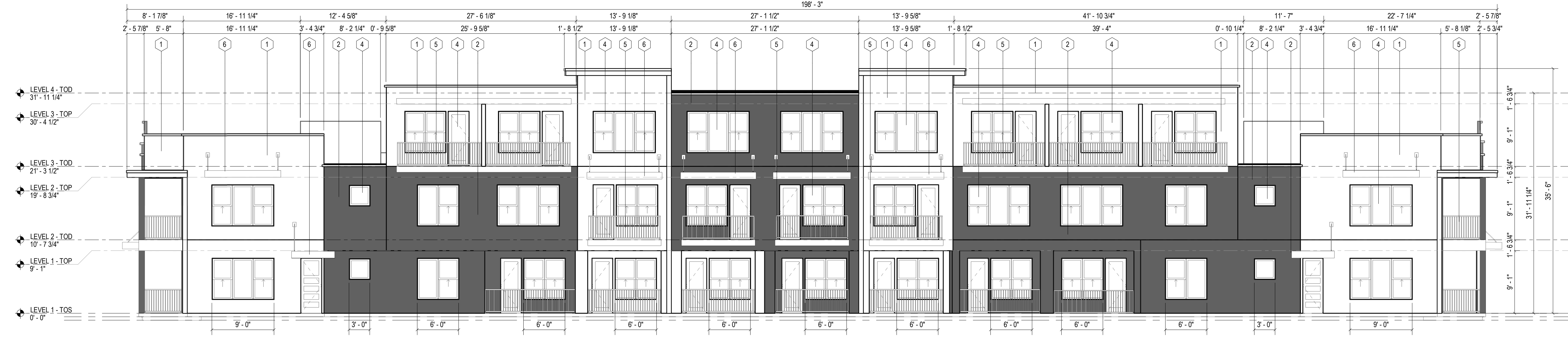
2 DRB - BLDG TYPE II - REAR ELEVATION 1/8" = 1'-0" 0 2 4 8 16
