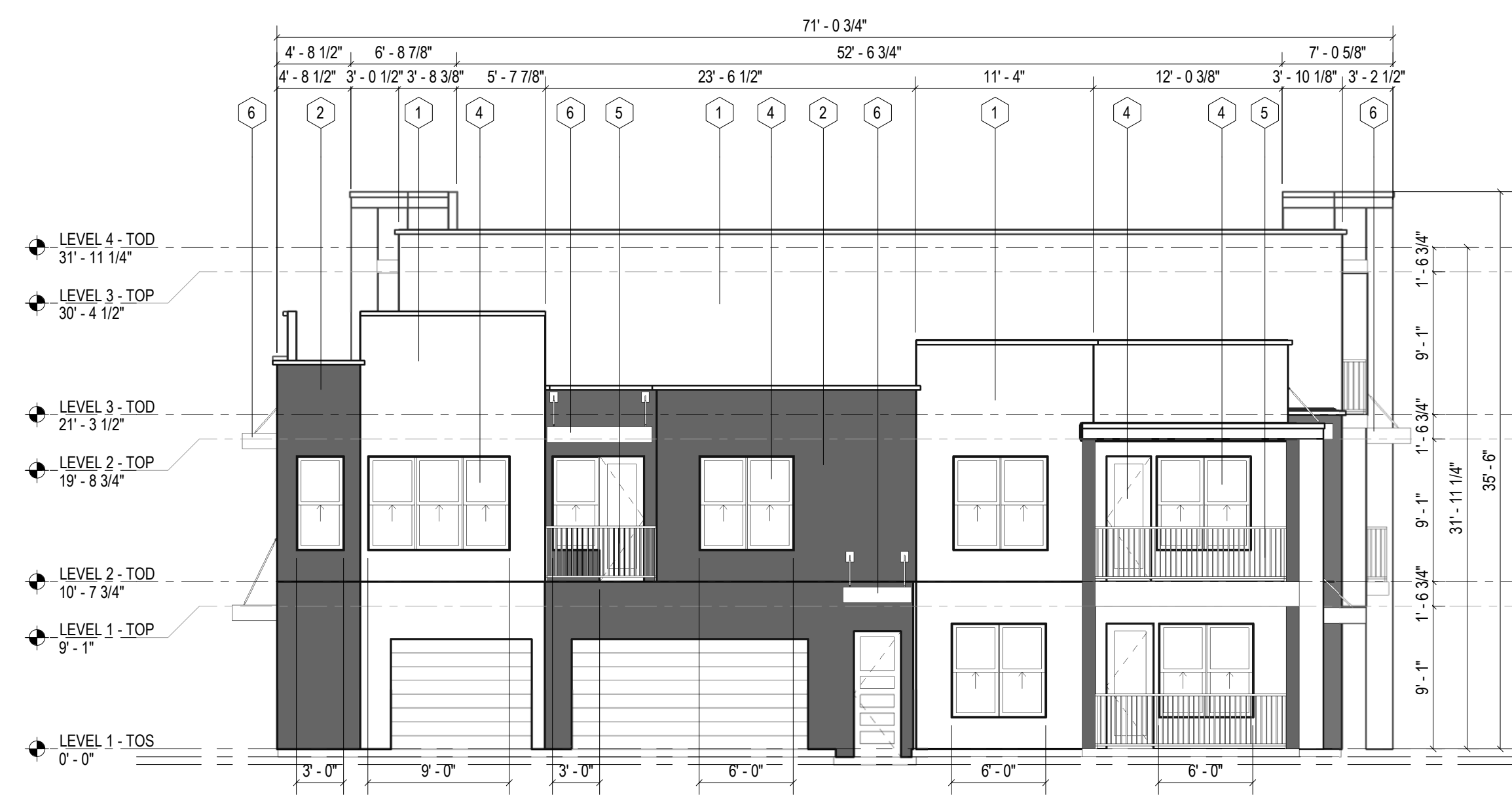
4 DRB - BLDG TYPE II - RIGHT ELEVATION 1/8" = 1'-0" 0 2 4 8 16
