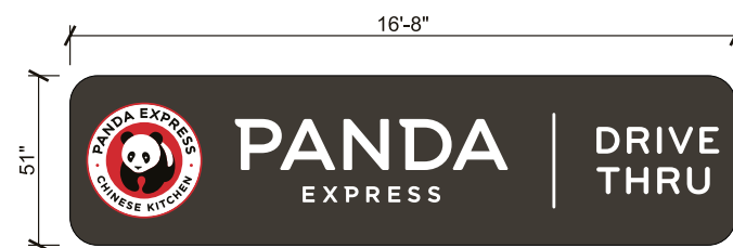
P1 Illuminated channel letters on panel Existing Double Poles Painted PMS Black 7C
