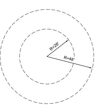
FIRE APPARATUS TURNING RADIUS
