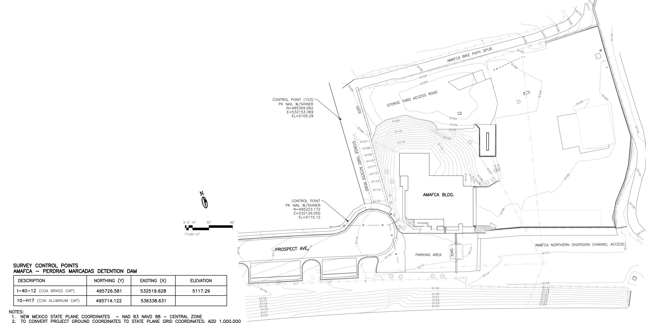
2. TO CONVERT PROJECT GROUND COORDINATES TO STATE PLANE GRID COORDINATES: ADD 1,000,000 TO THE NORTING AND EASTING THEN MULTIPLY GROUND COORDINATES BY 0.999672575
