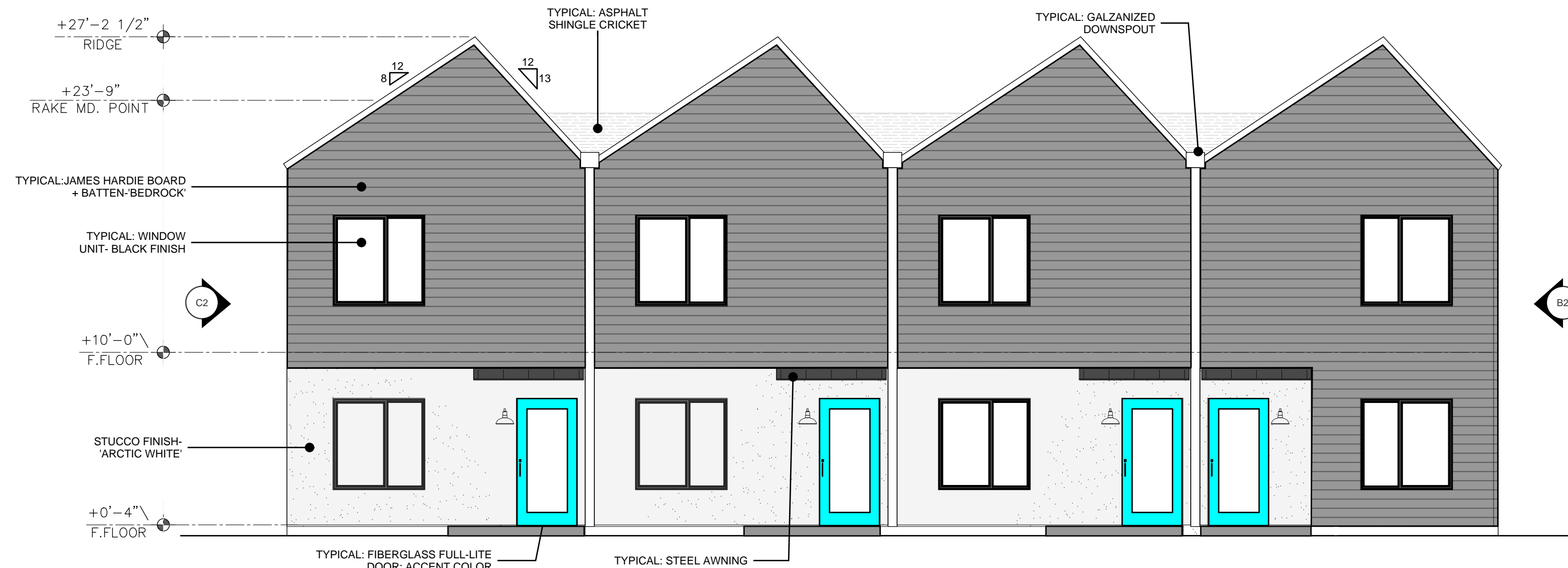
C1 TYPICAL FRONT ELEVATION 3/16"=1'-0"
