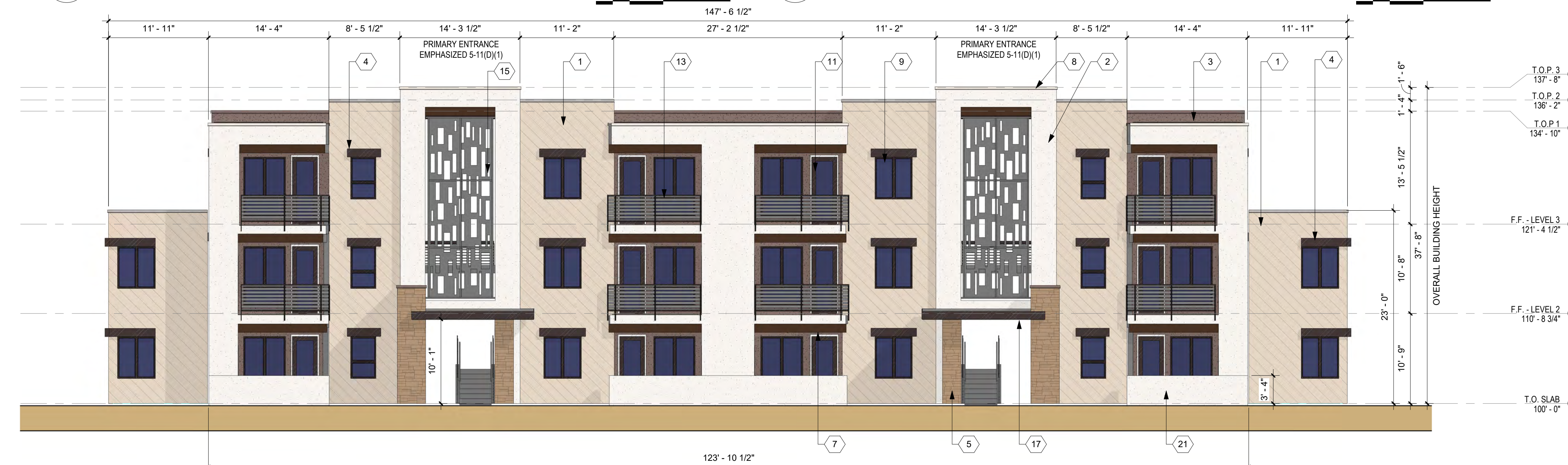
A1 BUILDING B WEST ELEVATION 1/8" = 1'-0"
