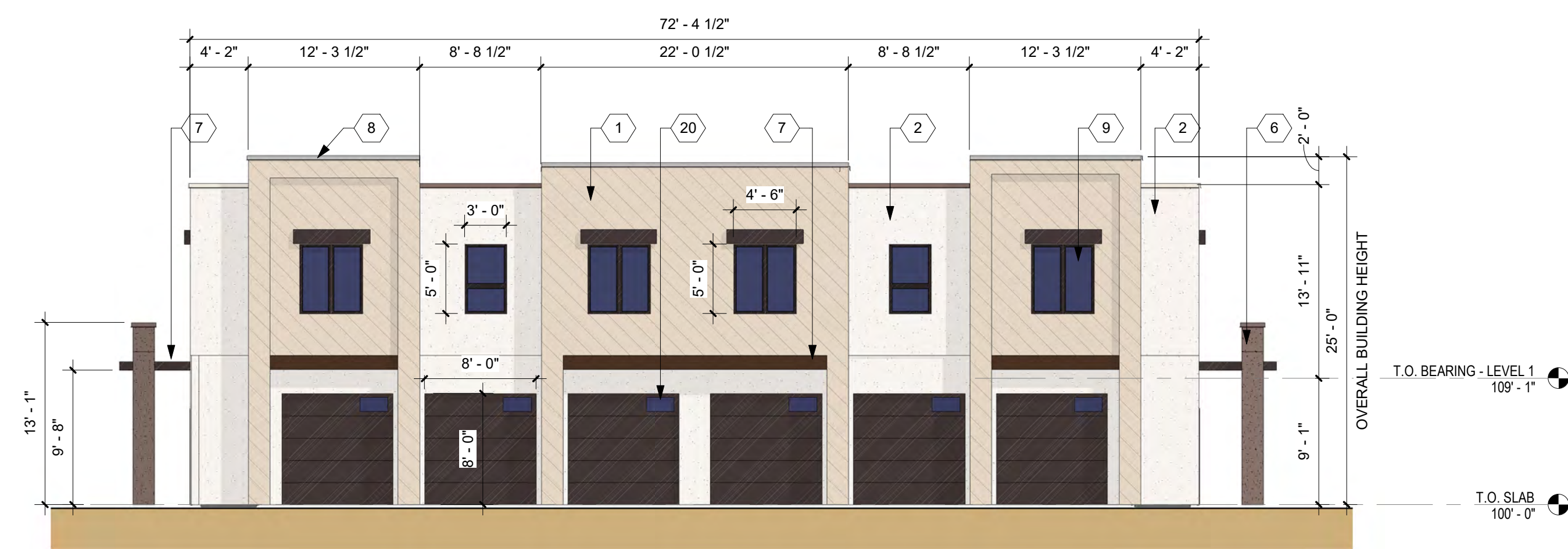
C1 BUILDING D - SOUTH ELEVATION 1/8" = 1'-0"
