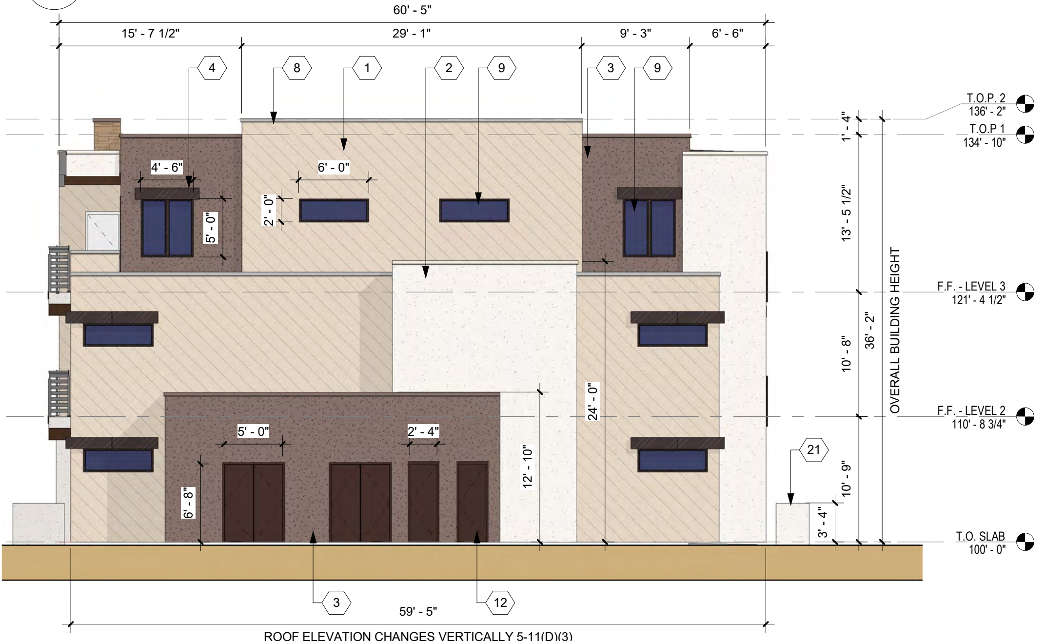
B1 BUILDING C WEST ELEVATION 1/8" = 1'-0"
