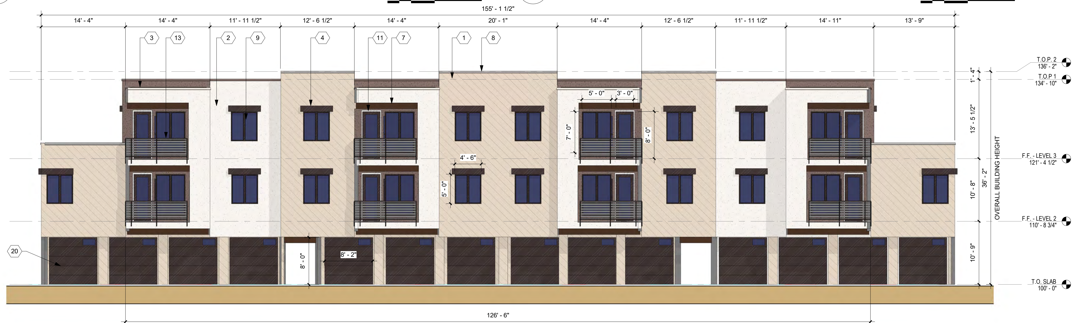
A1 BUILDING A NORTH ELEVATION 1/8" = 1'-0"
