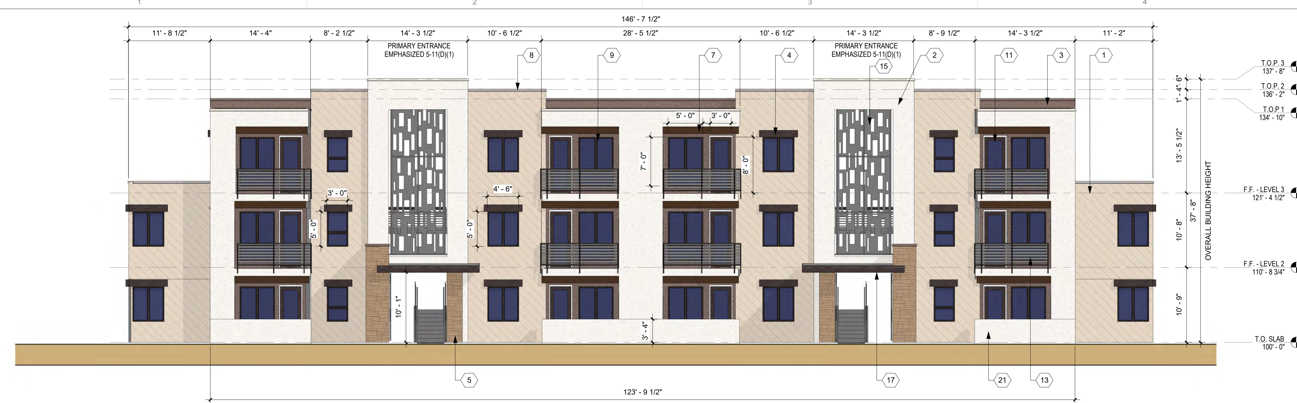
D1 BUILDING A SOUTH ELEVATION 1/8" = 1'-0"
