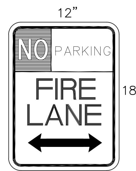
NO PARKING FIRE LANE SIGN
