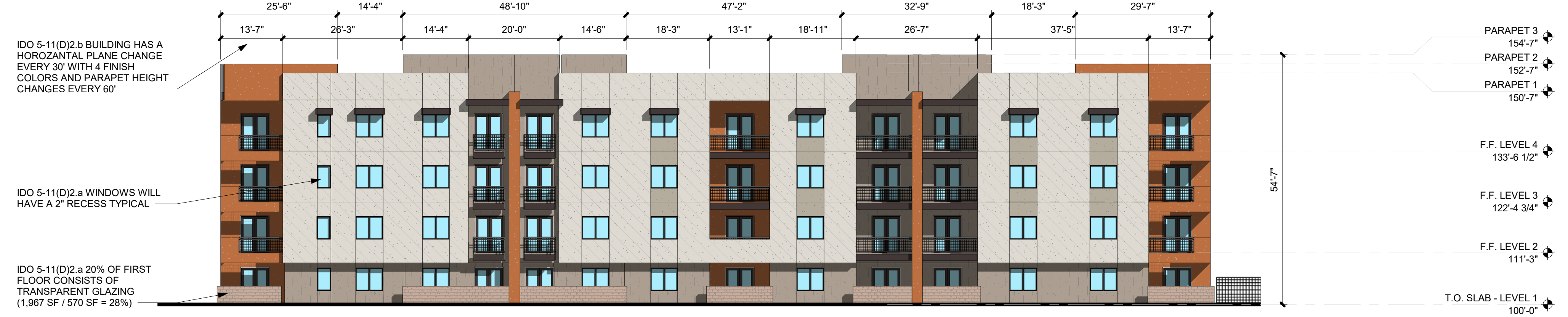
C4 BUILDING D - FRONT ELEVATION 1/16" = 1'-0" Scale: 1/16" = 1' - 0"
