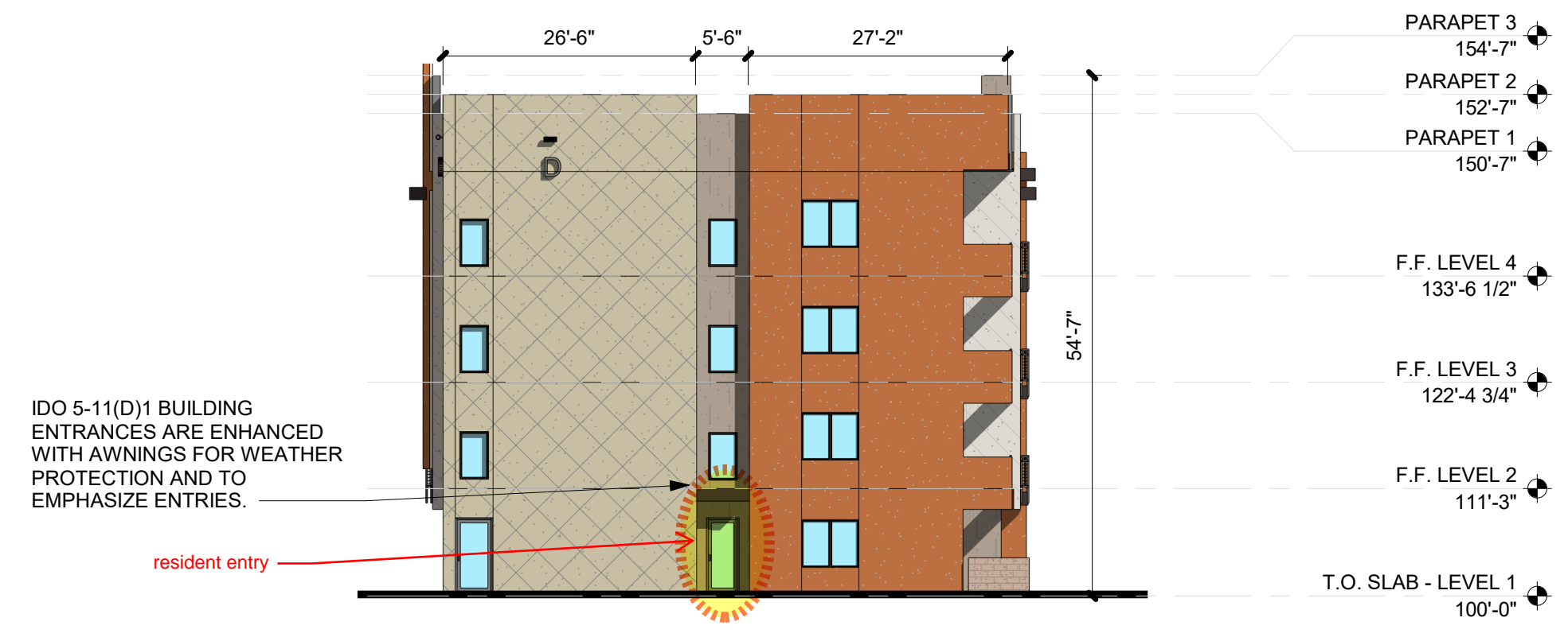
B2 BUILDING D - SIDE ELEVATION 1/16" = 1'-0" Scale: 1/16" = 1' - 0"
