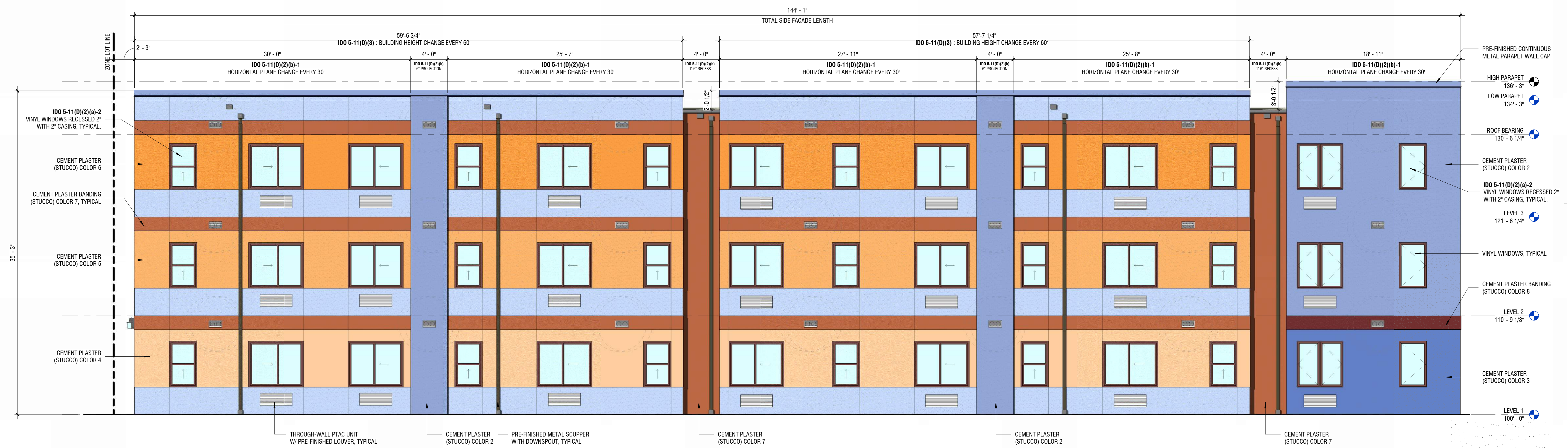
2 EAST ELEVATION (SIDE) 3/16" = 1'-0" 0' 4' 8' 16'
