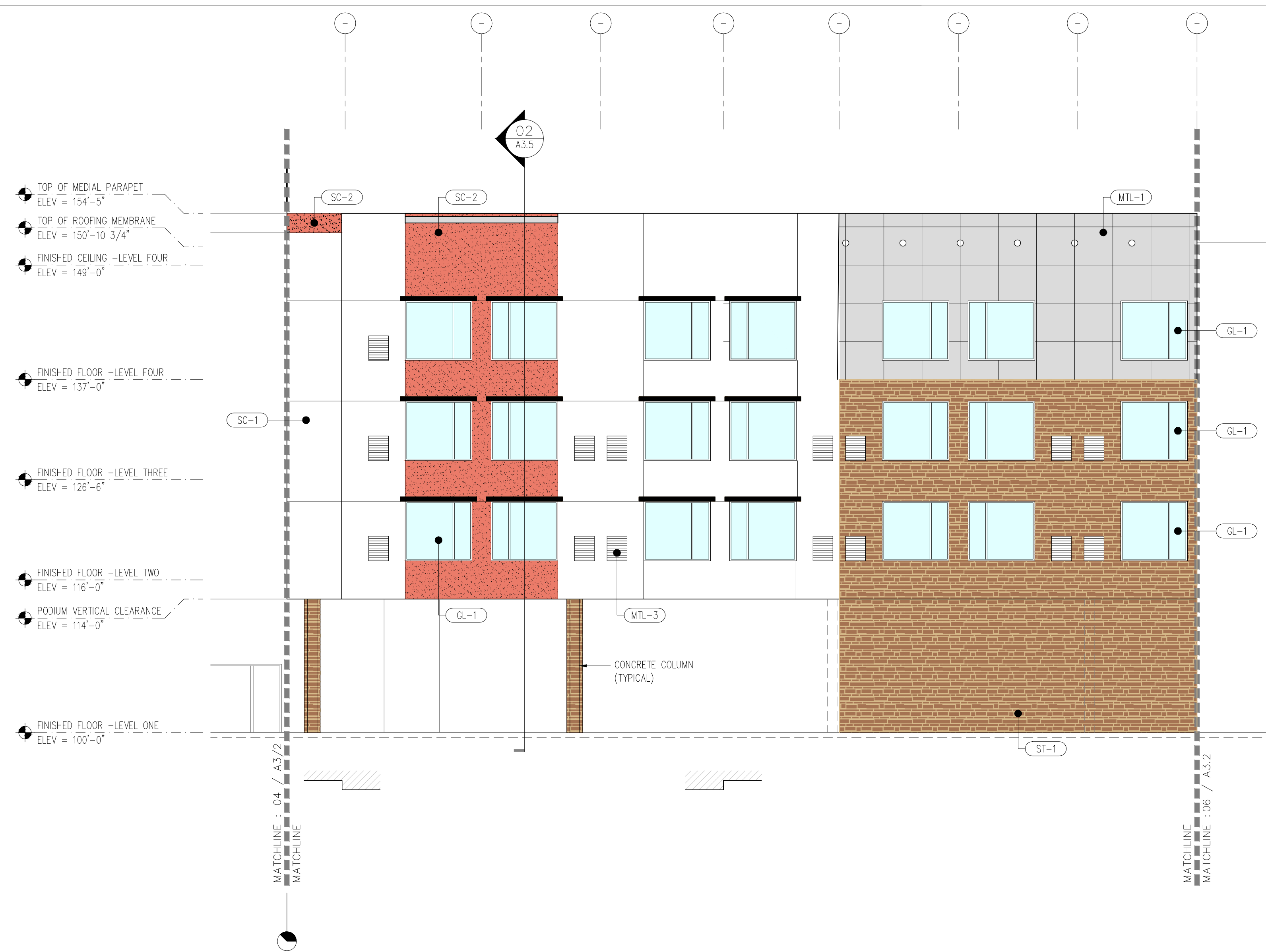
05 EXTERIOR ELEVATION WEST FACADE SCALE: 1/8" = 1'-0"
