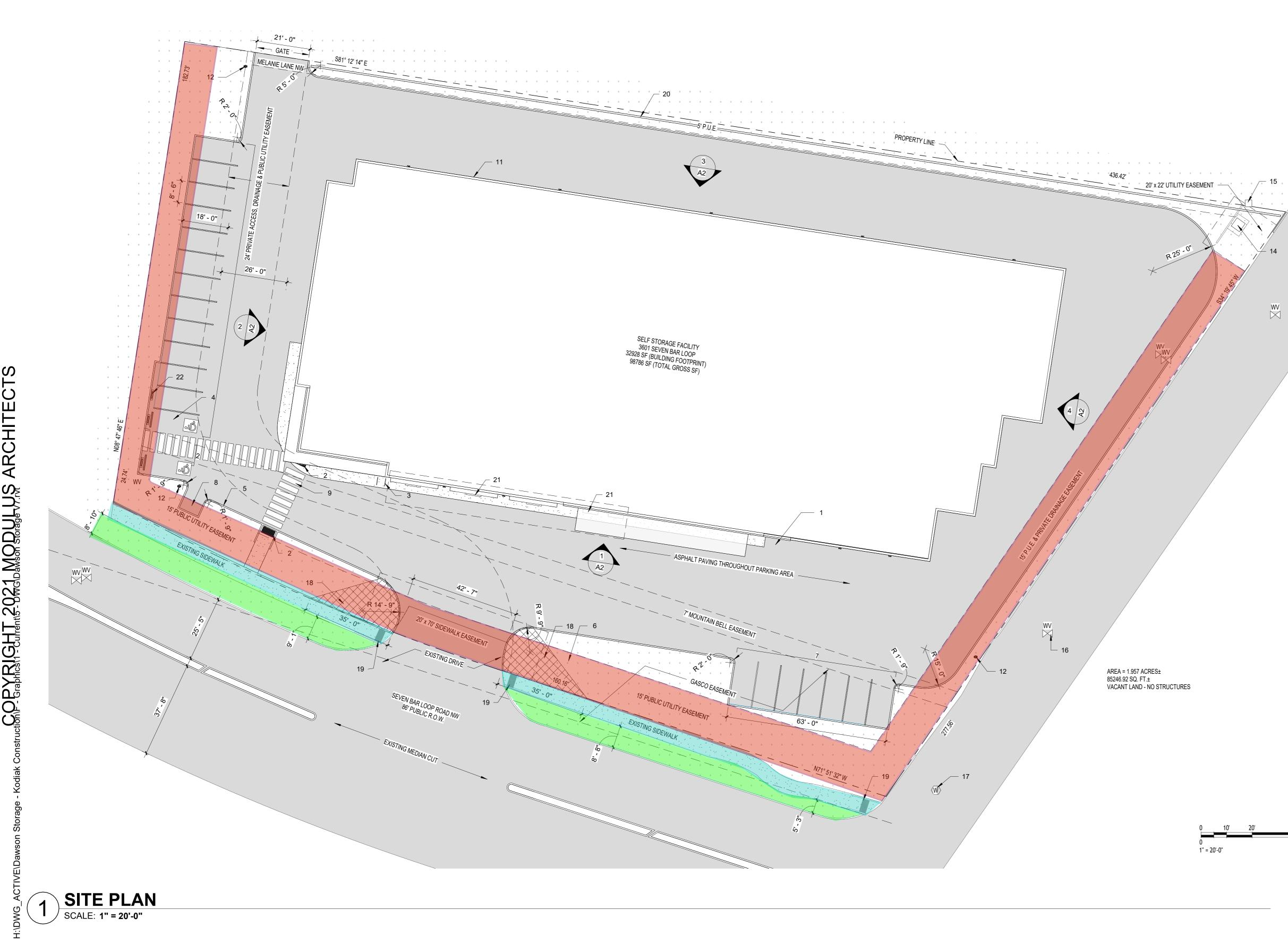
Sidewalk Waiver Area -The DPM requires 10' sidewalks along Seven Bar Loop and the most narrow point is 5' and the widest is 6'-4'. The sidewalk gradually widens going east and west of the access point. See attached exhibit. We are requesting a waiver to keep the existing sidewalks at the existing width.
