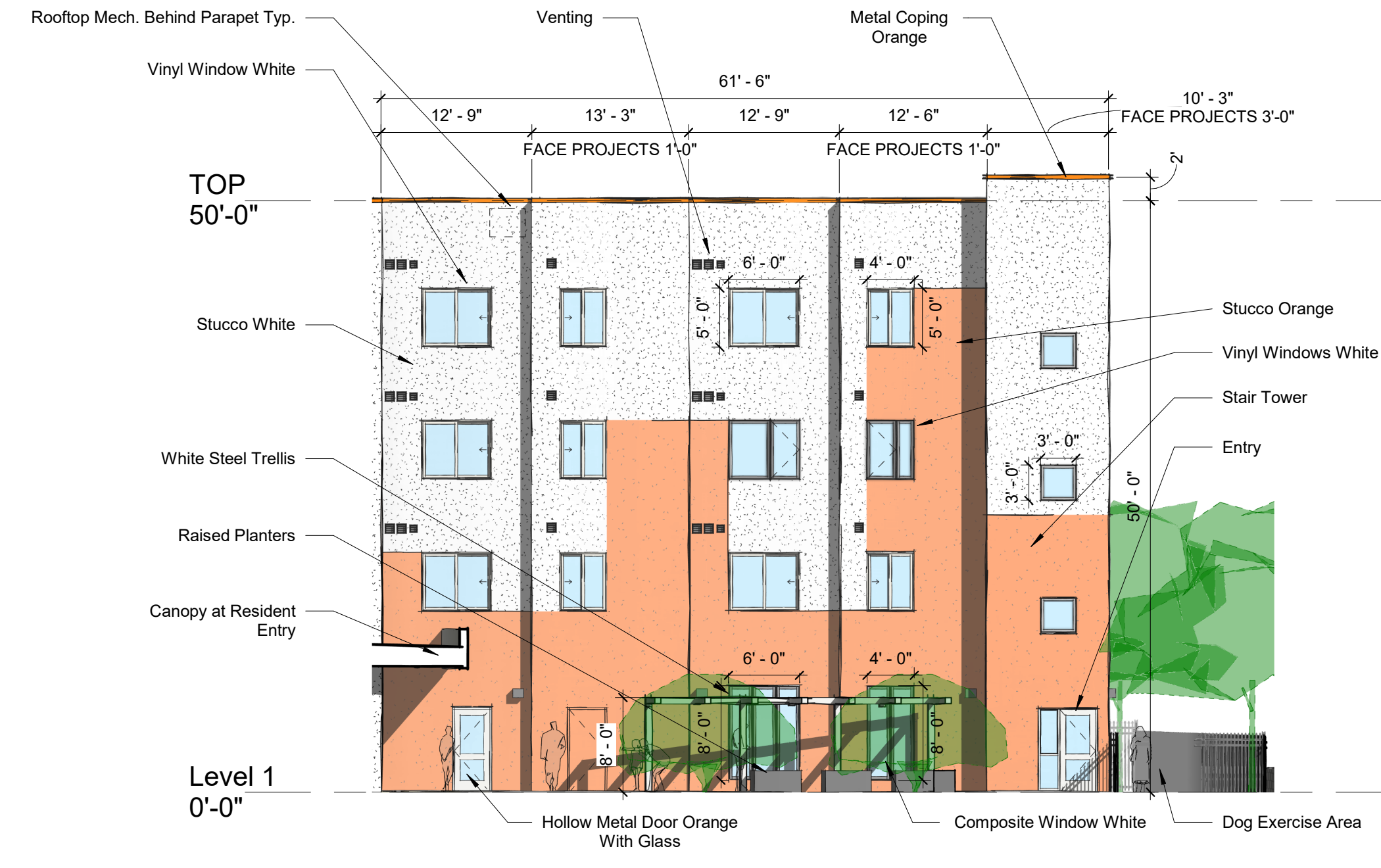
SOUTH ELEVATION (INTERIOR FACING FACADE) 3/32" = 1'-0"
