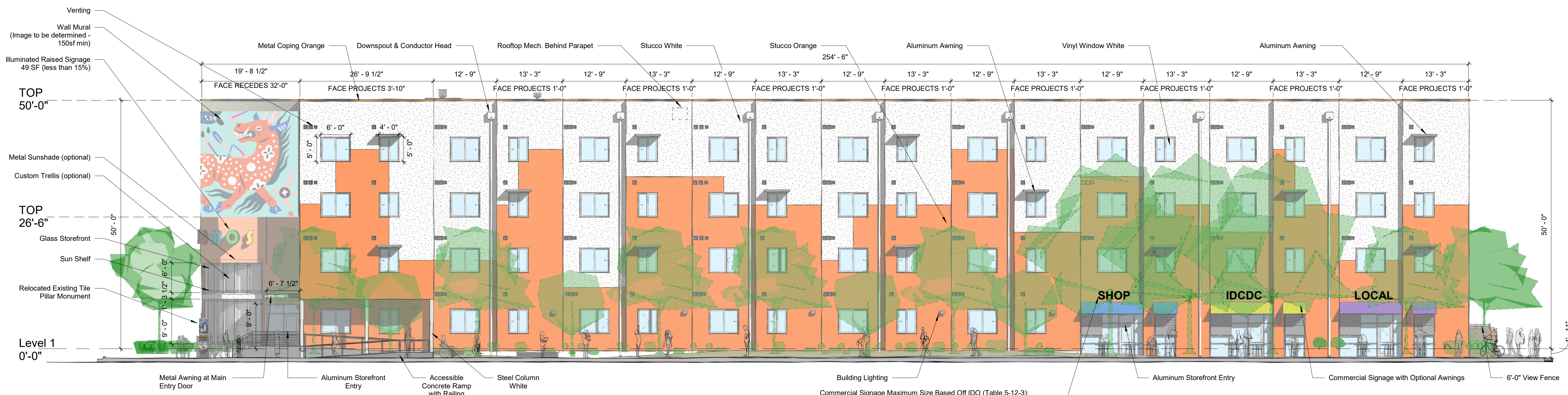
WEST ELEVATION (ALCAZAR STREET FACING FACADE) 3/32" = 1'-0"
