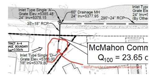
2. The proposed inlets, proposed storm pipes, and proposed manholes within McMahon R.O.W. along with the outfall into the Calabacillas Arroyo cannot be labeled as "By Others". All of this system is needed for this development and needs to be included in the Infrastructure List during the Preliminary Plat approval.
