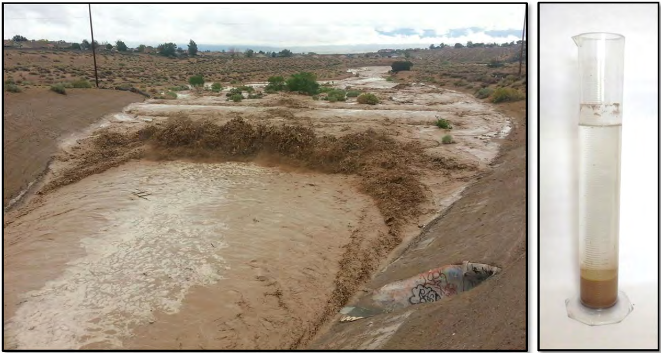
Photo 12: Sediment-laden stormwater runoff in the Calabacillas Arroyo downstream of Swinburne Dam (left), and a graduated cylinder showing the amount of sediment in a stormwater sample (right).
