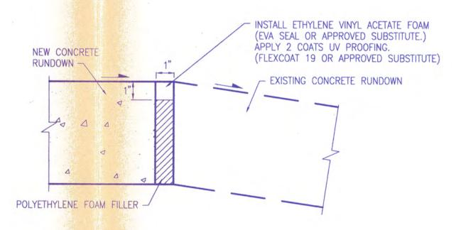
TYPICAL EXPANSION JOINT SECTION SCALE: 1" = 4"
