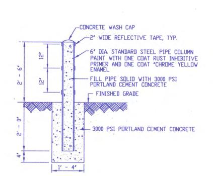
TYPICAL BOLLARD SECTION SCALE: 1' = 2' - 0'
