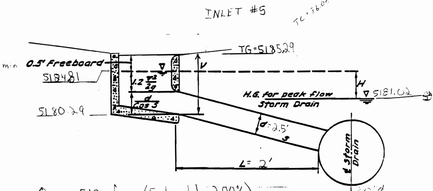
$$Q_{des} = 51.2 \text{ cfs} \quad (\text{Factored by } 200\%)$$
