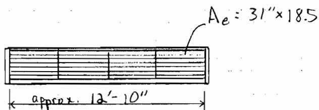
Capacity of Orifice (grate):
