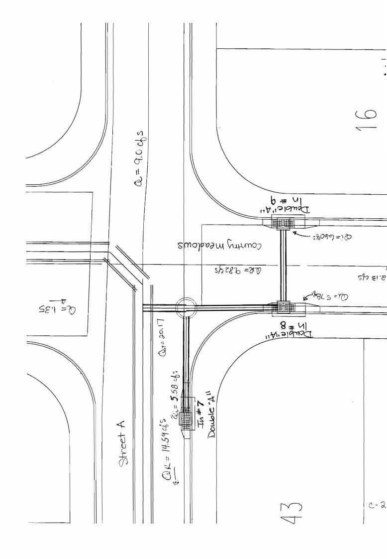
STREET A - INLETS 5&6 ANALYSIS OF AN INLET IN A SUMP CONDITION -
