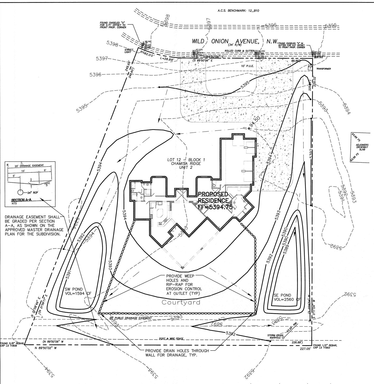
STANDARD GRADING NOTE: THE MAXIMUM GRADED SIDE SLOPE SHALL NOT EXCEED 3 FEET (HORIZONTALLY) TO 1 FOOT (VERTICALLY). AREAS DISTURBED BY GRADING WHICH WILL NOT BE TREATED WITH LANDSCAPING SHALL BE SEEDED.
