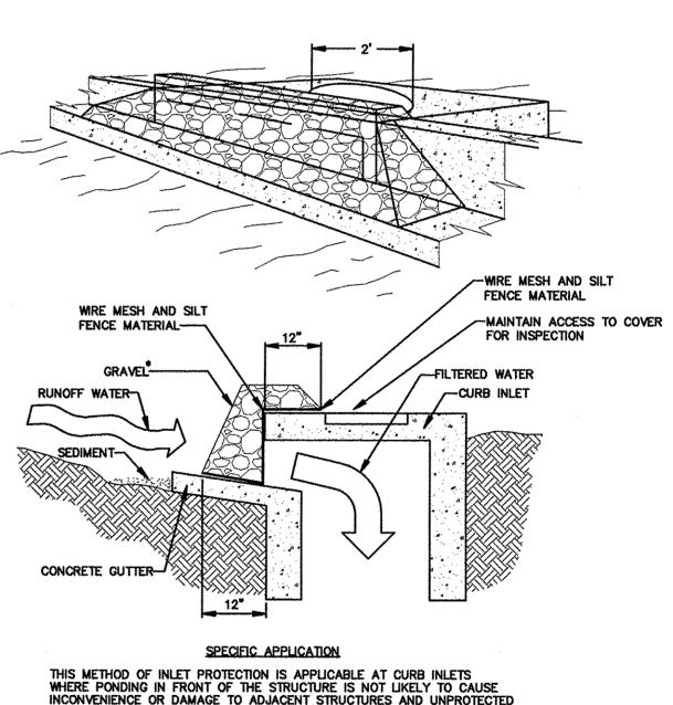
THIS METHOD OF INLET PROTECTION IS APPLICABLE AT CURB INLETS WHERE PONDING IN FRONT OF THE STRUCTURE IS NOT LIKELY TO CAUSE INCONVENIENCE OR DAMAGE TO ADJACENT STRUCTURES AND UNPROTECTED AREAS. \* GRAVEL SHALL BE 3/4"-2" ANGULAR CLEAN STONE
